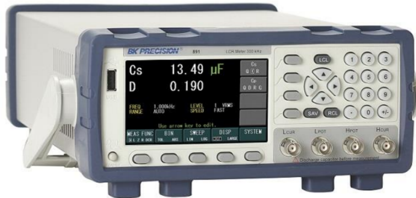
Figure 4.1. Impedance meter BK891.
