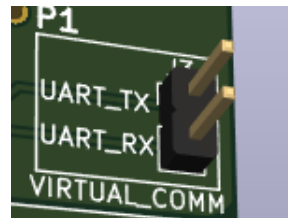
Figure 3.43: Pin Header Serial Console interface
