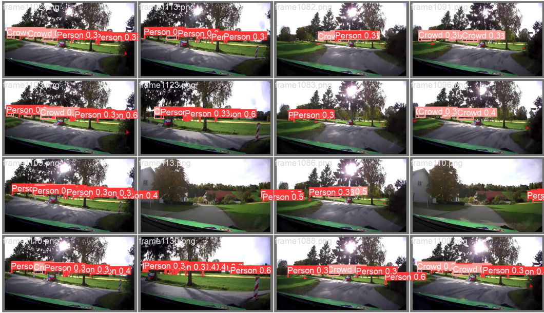
Figure 4.3: An example of 16 post-processed images batch, in which the predicted bounding boxes are drawn along with the respective label and a number representing the confidence of the prediction.
