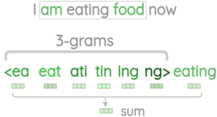
Figure 2.4: FastText sub-word representation using the word "eating" as example.
