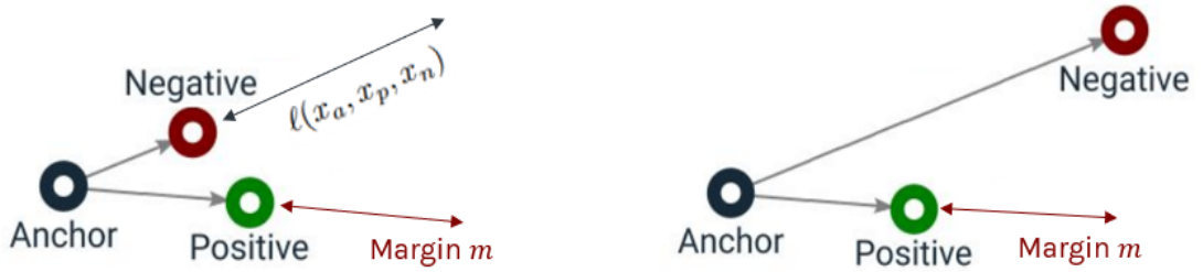
Figure 4.14: Triplet Loss visual representation. The image representations of the positive p and the anchor a are pulled together in the latent space while the representation of the negative n and the anchor one a are pushed away enforcing the margin m_n .
