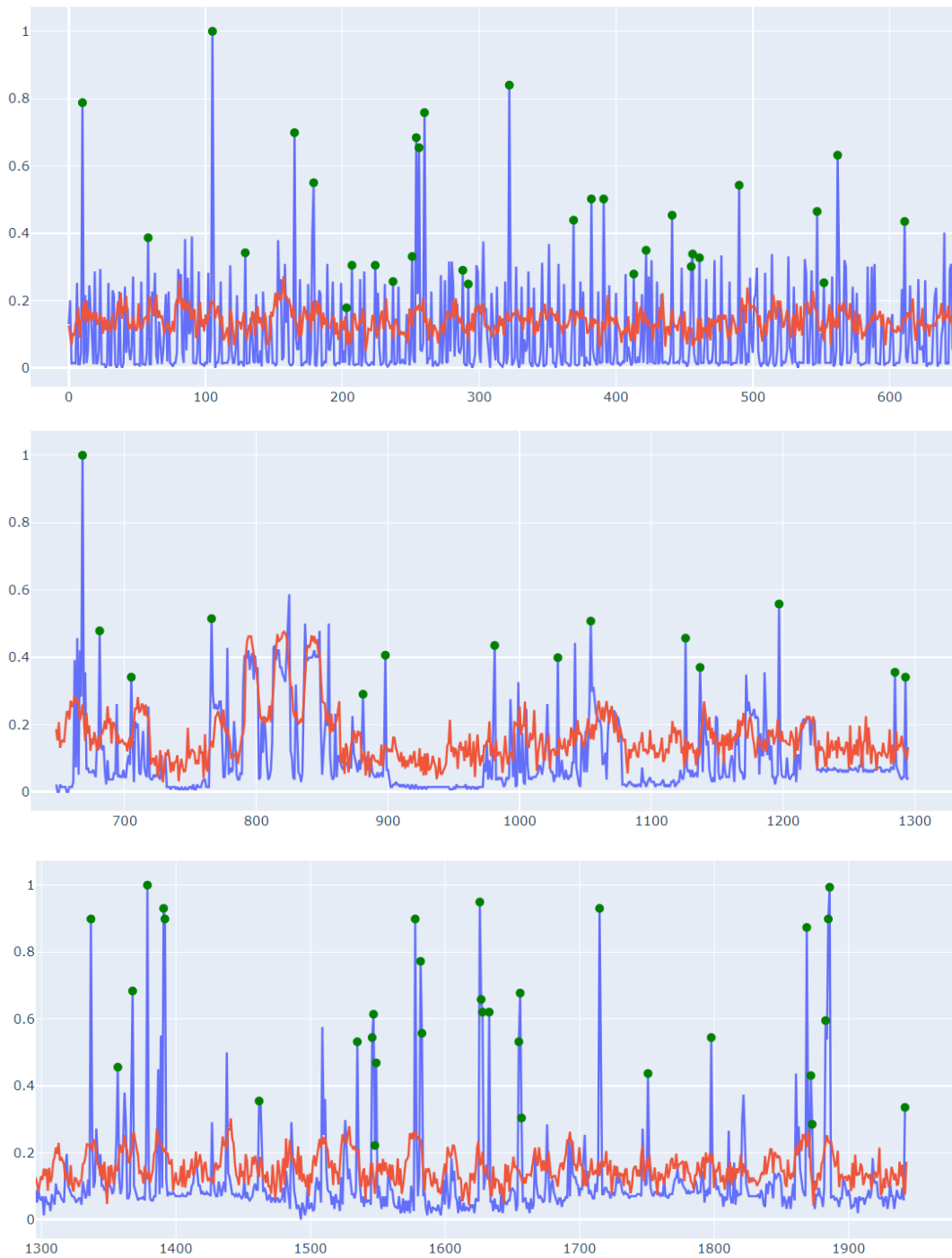
Figure 4.8: Examples of reconstructions of three time series from 2021 using LSTM Autoencoder. In blue the original input, in red the reconstruction, in green the anomalies as identified with Method 3
