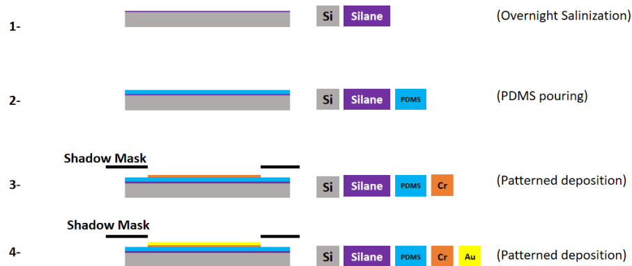
Figure 6.1: PDMS-Au electrodes fabrication process
