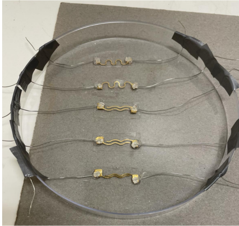
Figure 6.6: Electrodes with silver paste and silicon layers in the pads position while drying.
