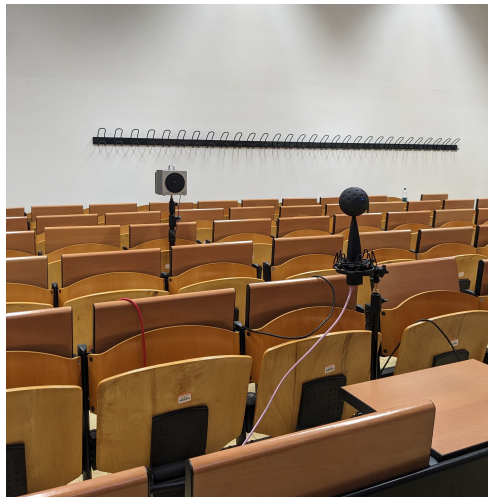
Figure 4.26: Representation of the first set of Inter-ASL measurements for collecting acoustic scenes. The Eigenmike is positioned at R1, and the talkbox at S3.
