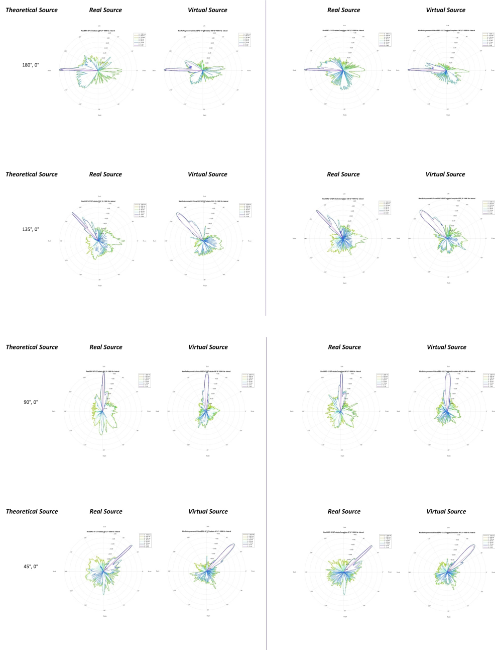
Figure 4.10: Lateral polar diagrams at 0° elevation and azimuths of 180°, 135°, 90°, and 45°, for both real and virtual environments at 1000 Hz frequency, illustrating laboratory acoustic conditions with the first treatment condition (left) and the second treatment condition (right).
