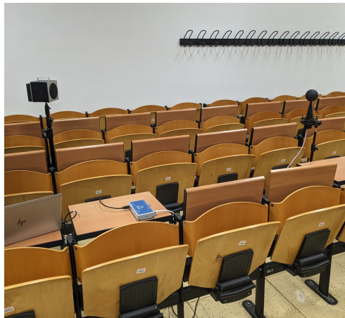
Figure 4.28: Representation of the second set of Inter-ASL measurements for collecting acoustic scenes. The Eigenmike is positioned at R2, and the talkbox at S4.
