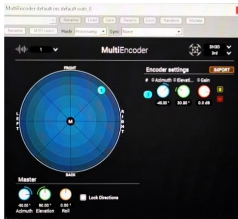
Figure 4.6: Multi-Encoder plugin of the Bidule software, allowing you to set the azimuth and elevation of the desired sound source.
