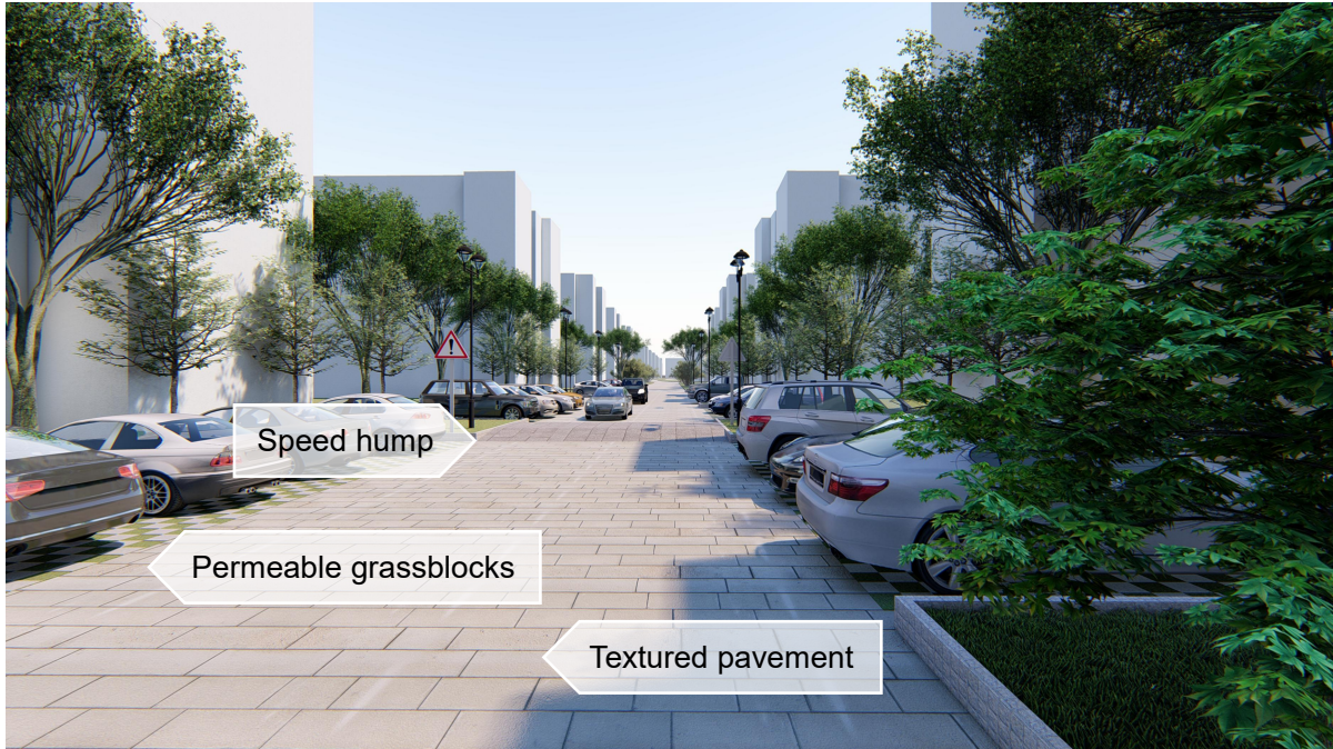
Figure 6-31: Improvement schematic of group road in Diewu Xuan
