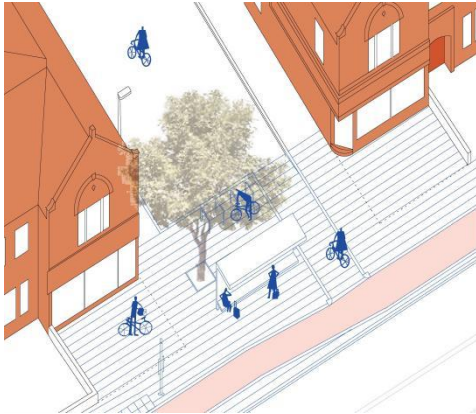
Figure 3-15: Modal filter on Kettlebaston Road
