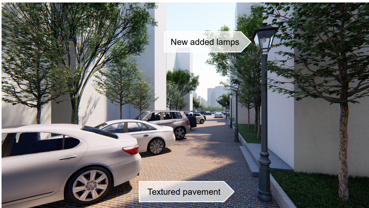
Figure 6-32: Improvement schematic of house road in Lvyi Ju
