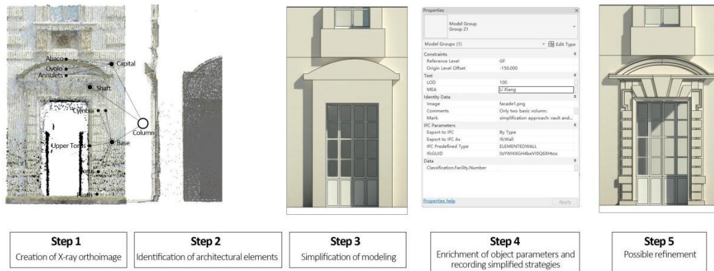
Figure 30 A simplified modelling approach for the door and its surroundings
