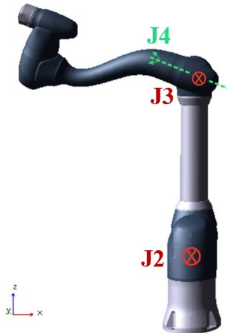
Figure 43 Initial condition of Joint 3 and Joint 4 set to 70^\circ
