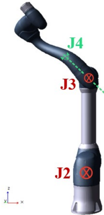
Figure 42 Initial condition of Joint 3 and Joint 4 set to 40^\circ
