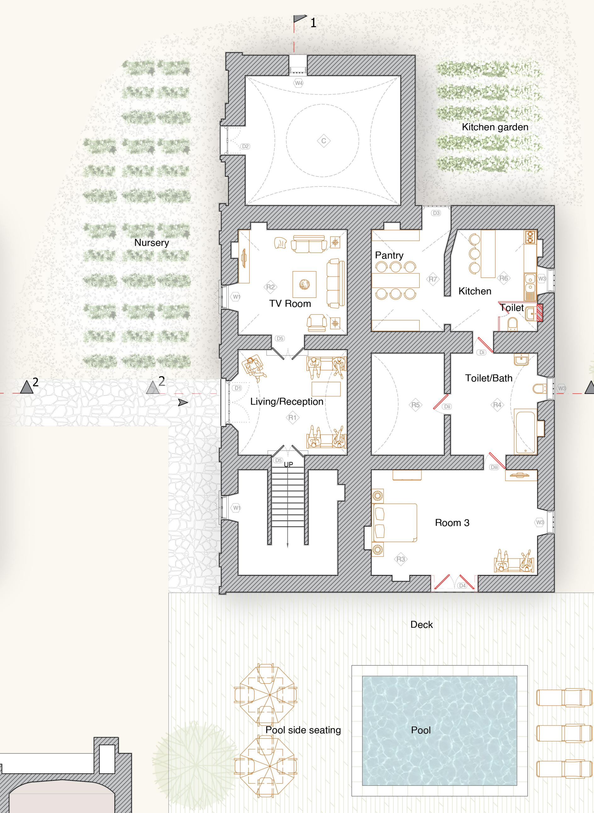
Ground floor plan 1 : 100
