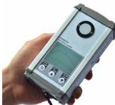
Figure 3.9. “BTS256-EF for complex measurements in lighting technology, including flicker measurement”.
