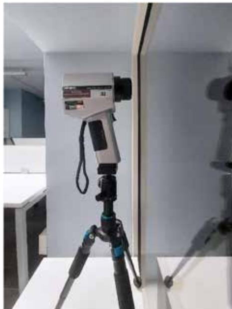
*Figure 3.12. Field measurement with a Luminance Meter Konica Minolta LS-100.*
