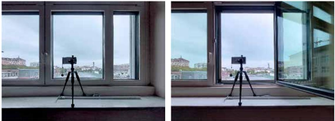
Figure 3.8. Measuring process to calculate light transmittance.
