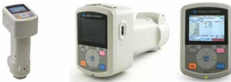
Figure 3.11. Contact spectrophotometer Minolta M-600. Photos from *konicaminolta.us*.
