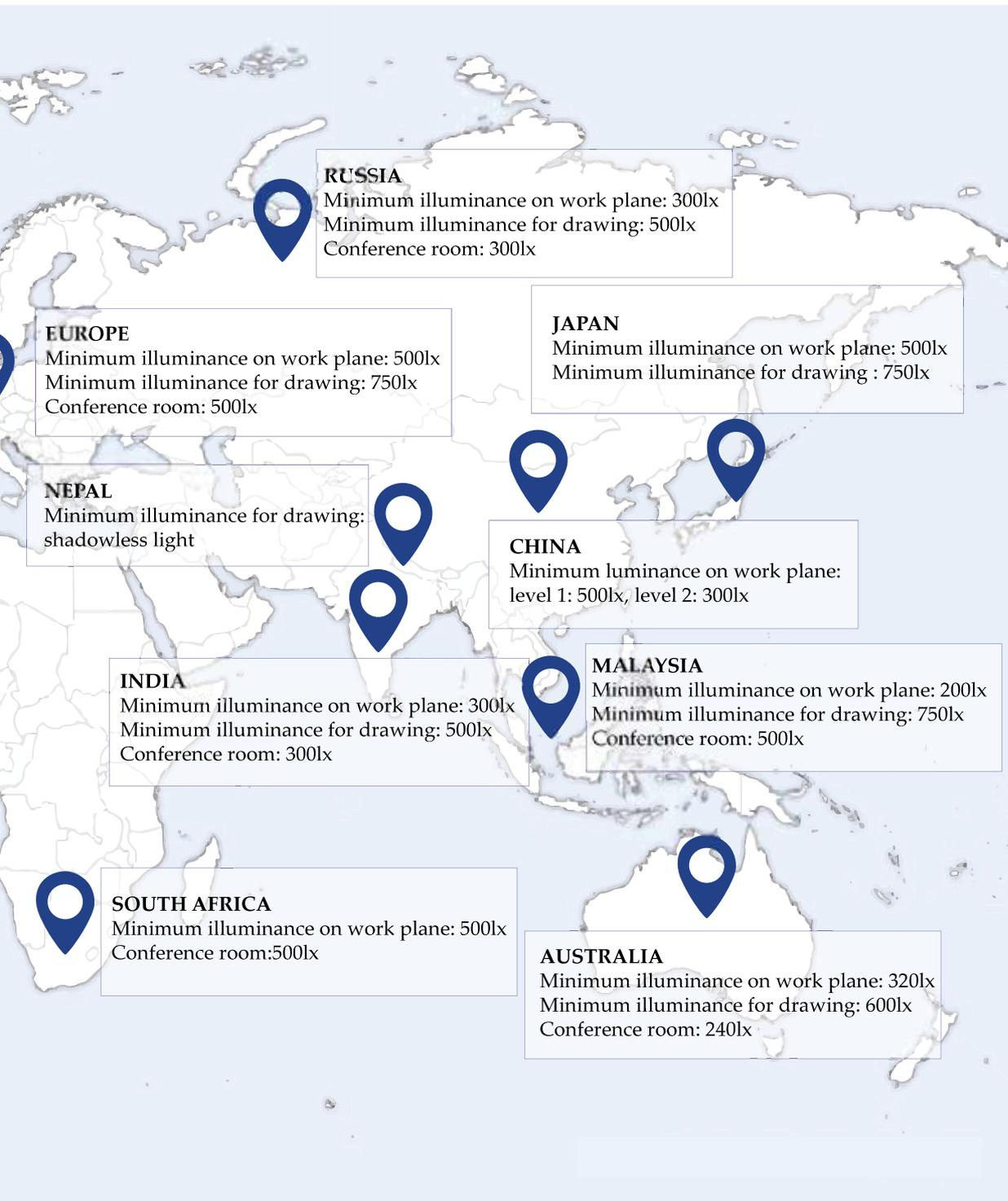
Figure 4.4. Minimum illuminance on work plane (horizontal) for drawing and minimum illuminance on conference rooms. From Martinsons C., (2010), Guidebook on Energy Efficient Electric Lighting for Buildings.
