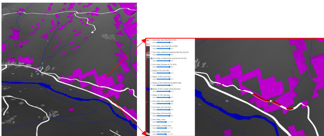
Figure 88. Slope terrain percentage between 35 and 70%. Streets and buildings at risk of complex terrain movements (35-70%) in red.
