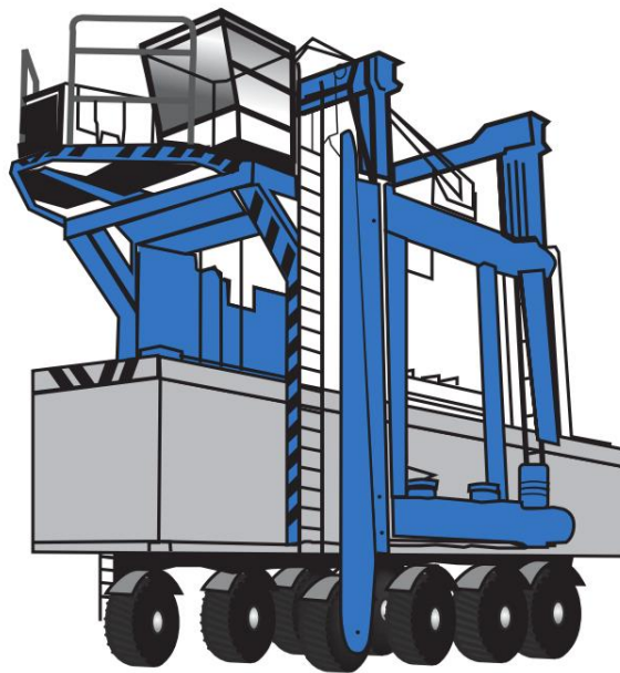
Figure 3.1.3: Container straddle carrier (Knapton, 2008)
