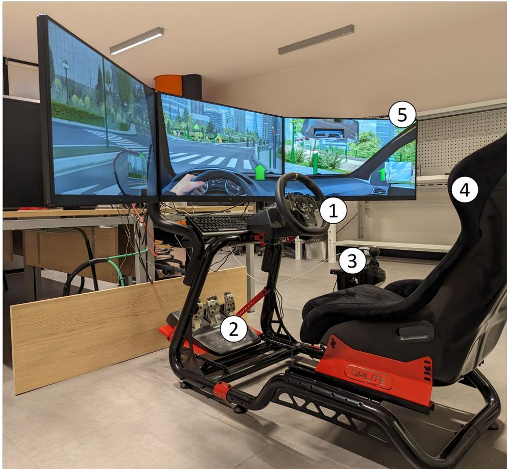
**Figure 1.1:** Driving simulator paired with SCANeR™Studio. 1: force feedback steering wheel, 2: pedals, 3: manual gearbox, 4: bucket seat, 5: high resolution screens.
