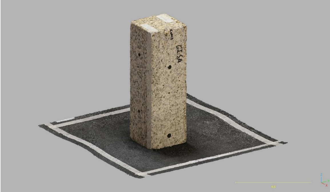
Figure 3.1 3D model of Specimen A generated using photogrammetric techniques. Units in meters.
