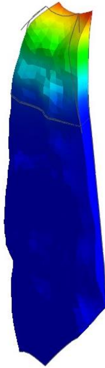
Figure 4.21 Eigenfrequency analysis result for the unstable block only.
