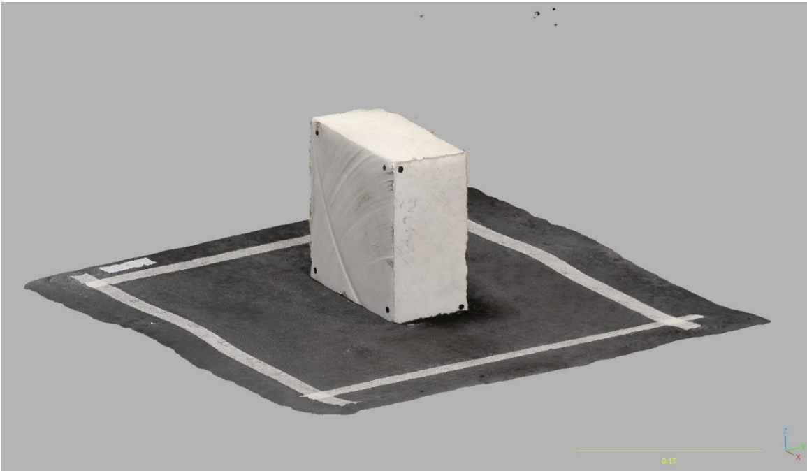
Figure 3.2 3D model of Specimen B generated using photogrammetric techniques. Units in meters.
