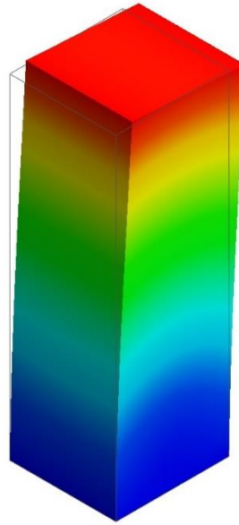
Figure 3.14 Second eigenmode displacement visualization in GTS NX for Specimen A.
