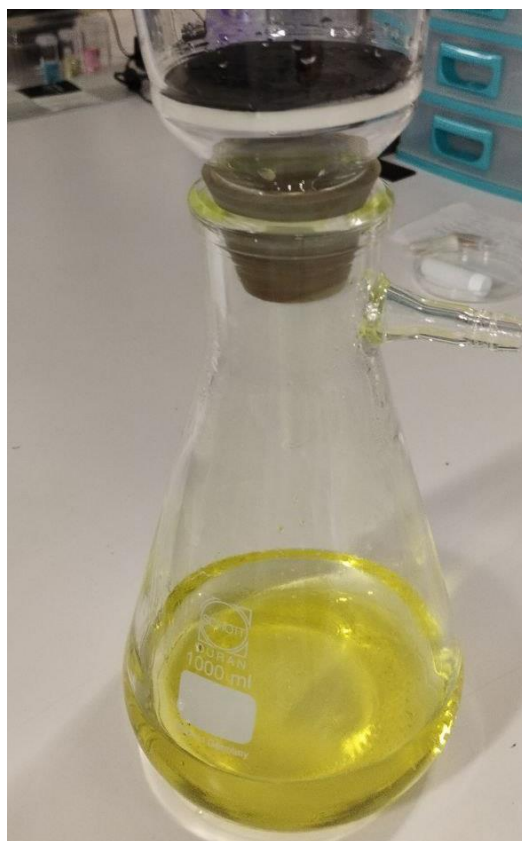
Figure 13. Catalyst filtration after HCl etching.
