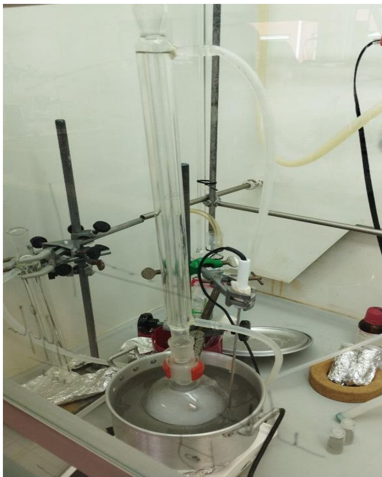
Figure 10. Solvent extraction with a condenser on top.
