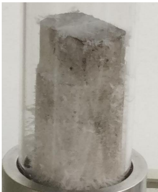
Figure 33. 1,10-phenanthroline crystallised at the bottom of the pyrolysis reactor.
