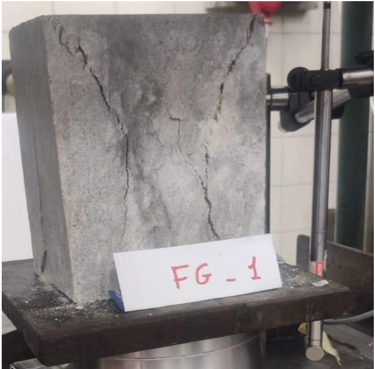
Figure 34 shows the failure of specimen after testing
