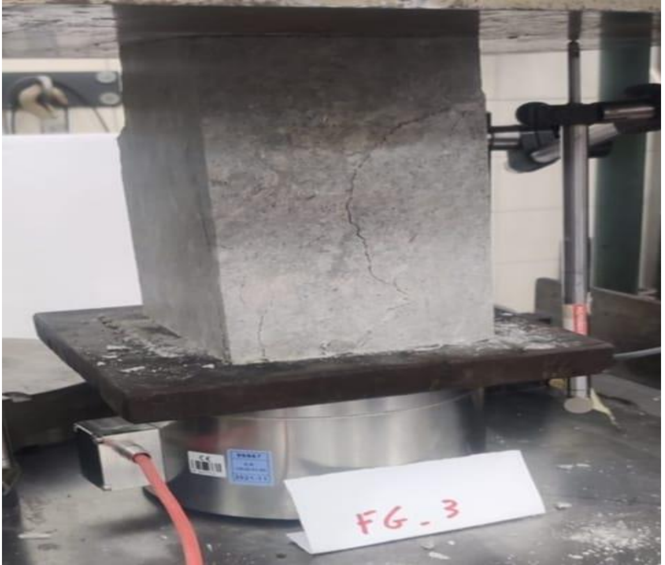
Figure 40 shows the failure of specimen after testing
