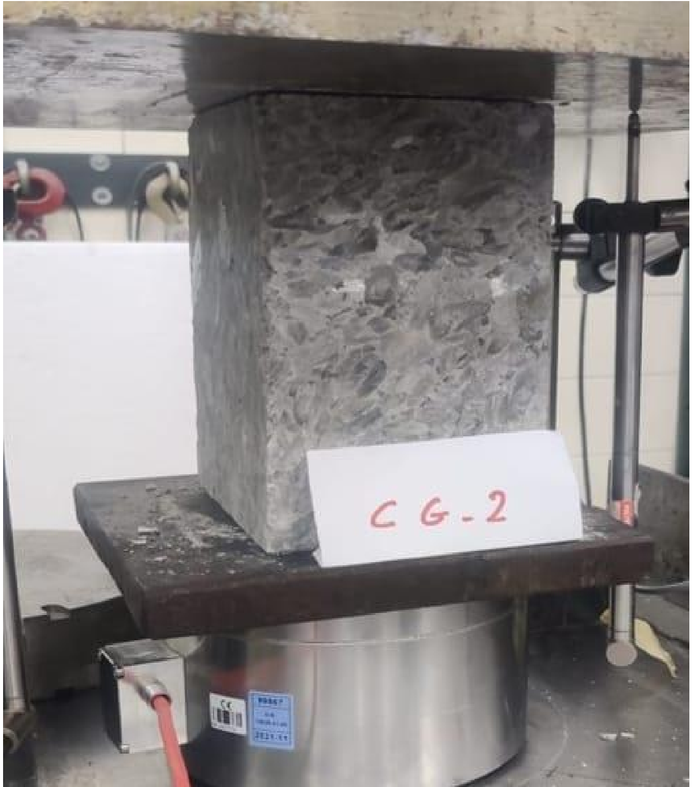
Figure 44 shows the testing procedures performed on sample coarse grained specimen 02 From the stresses and strains we have obtained the following results.
