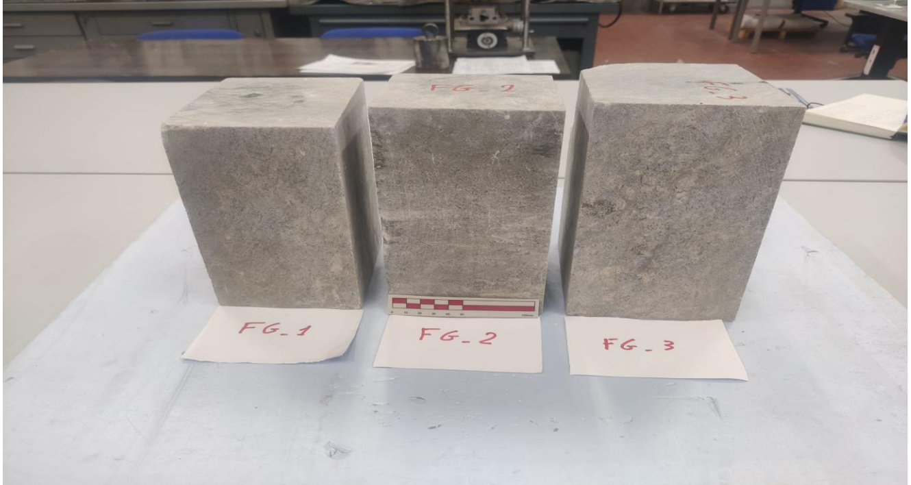
Figure 30 shows the fine grained specimens of gypsum obtained from the samples, on which testing have been performed.
