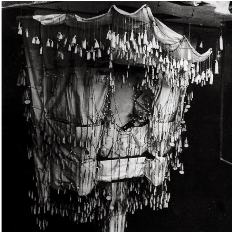
Figure 6: Hanging model for the Sagrada Familia
