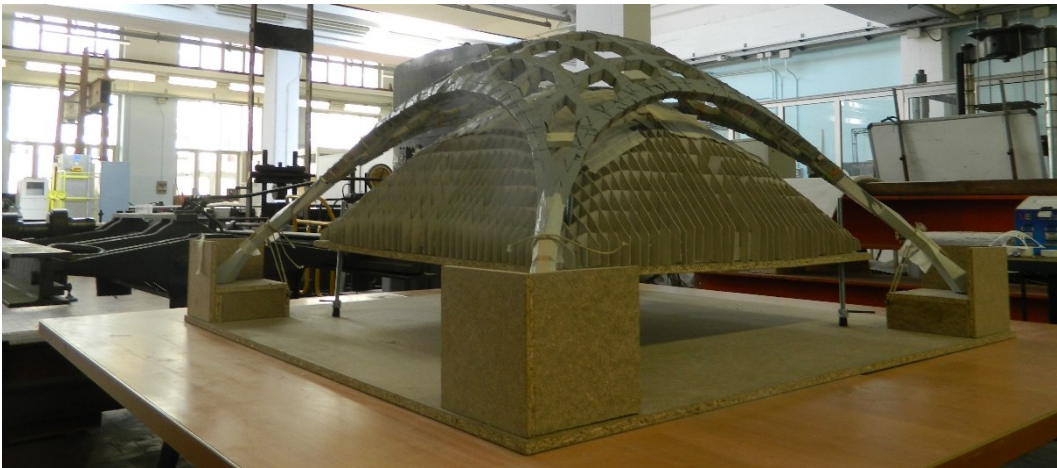
Figure 92: The ended prototype during falsework removal phase – picture 2
