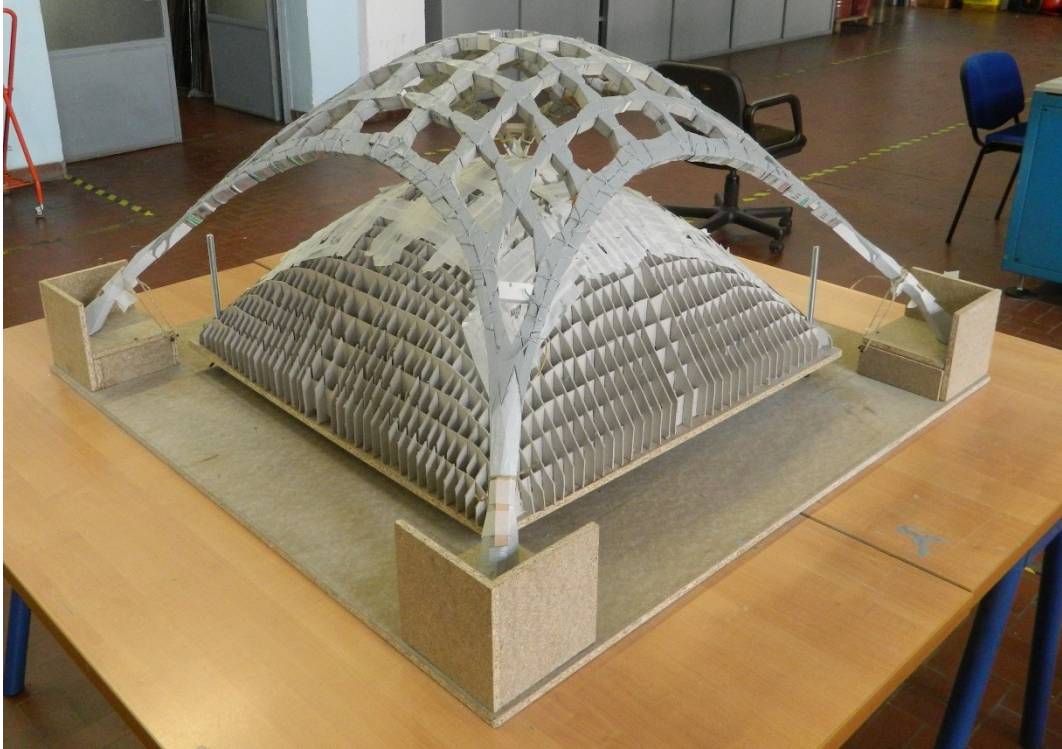
Figure 94: The ended prototype during falsework removal phase – picture 4
