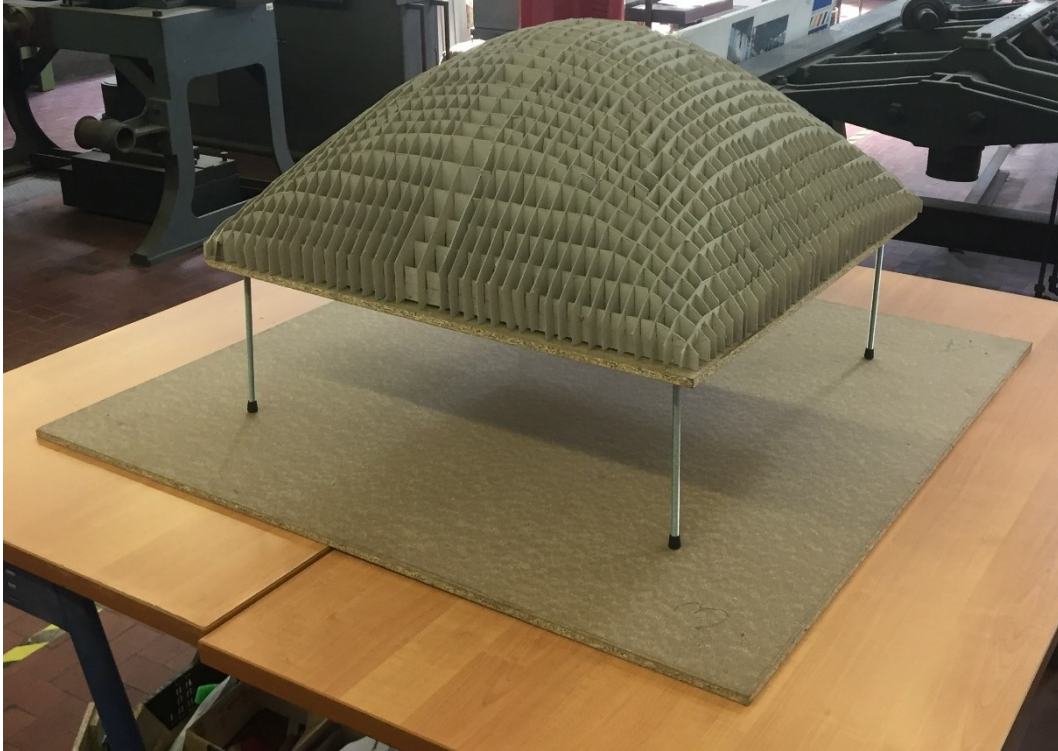
Figure 73: the falsework positioned on the plywood panel supported by 4 threaded bars
