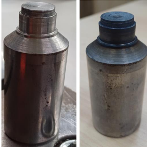
Figure 10. Dwelling time 10 s: Tool before (left) and after (right) the set of trials.
