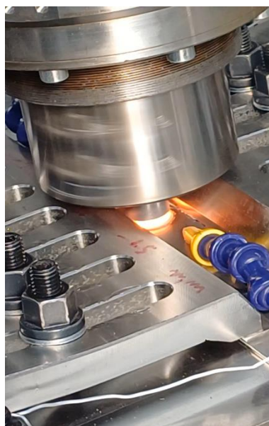
Figure 7: Image depicting the joint creation during the dwell phase.
