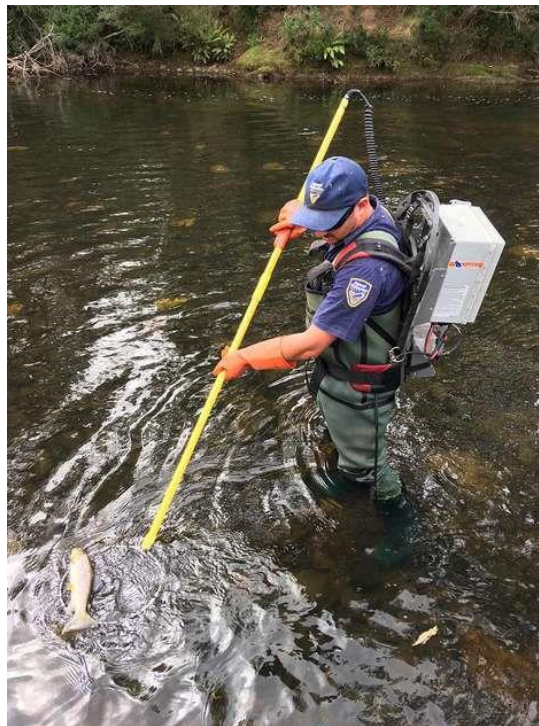
Figure 31: Electric Fishing Instrument (Tasmanian Government, 2018)
