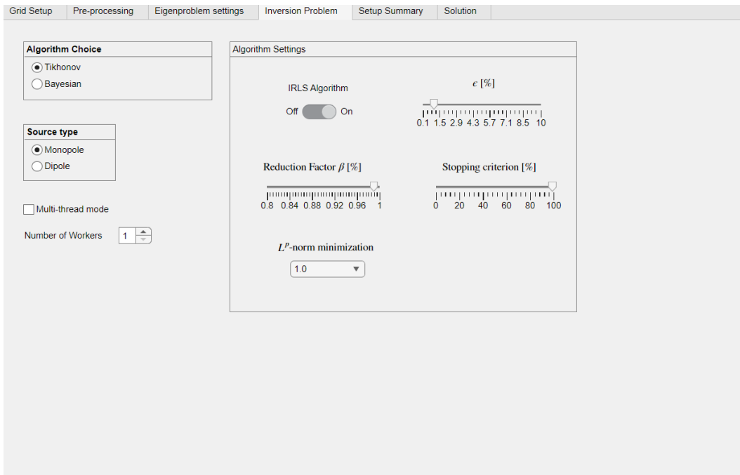
Figure 5.4: View of the inversion problem tab, where the user can indicate the IRLS parameters.
