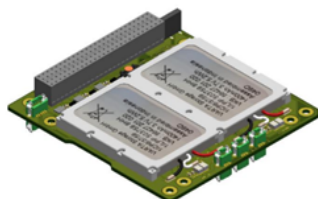
Figure 4.10: Electrical Power Supply [41]
