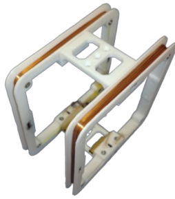
Figure 5.8: Single-axis Helmholtz Cage Reference Project
