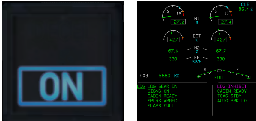
(a) Maschera Auto BRK LOW ON (b) Checklist aggiornata Auto BRK LOW
