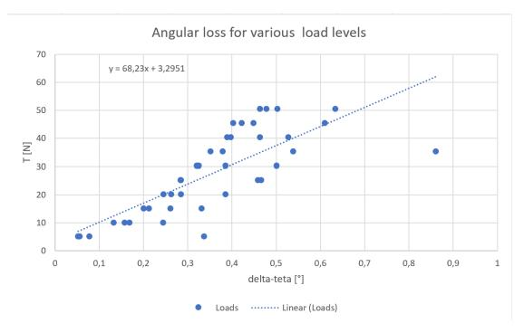
Figure 5.11: Angular loss for various load levels
