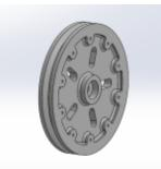
Figure 4.10: Pulley (CAD)
