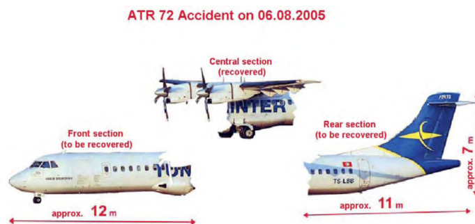
Figure 4.11: Case 2: How the aircraft broke down
