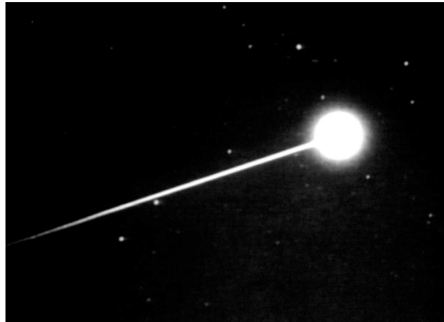
Figure 1.1: Dr. Mike Taylor (Utah State University) got a spectacular video sequence of the Stardust capsule re-entry onboard the DC-8 aircraft using a Xybion intensified camera. Credits: Dr. Mike Taylor. [3]
