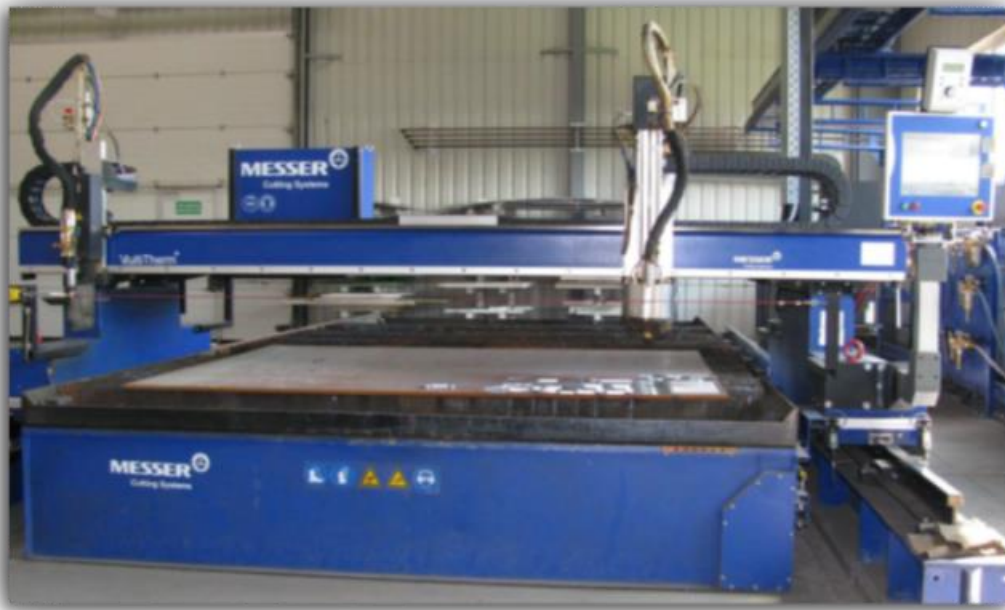
Figure 4: MESSER Multitherm 4000 Plasma Cutting Machine- 3 axis
