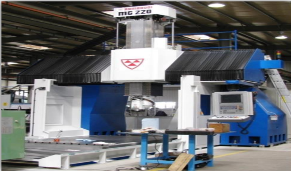
Figure 5: Rambda MG 220 – 3 axis- for machining operation as well
