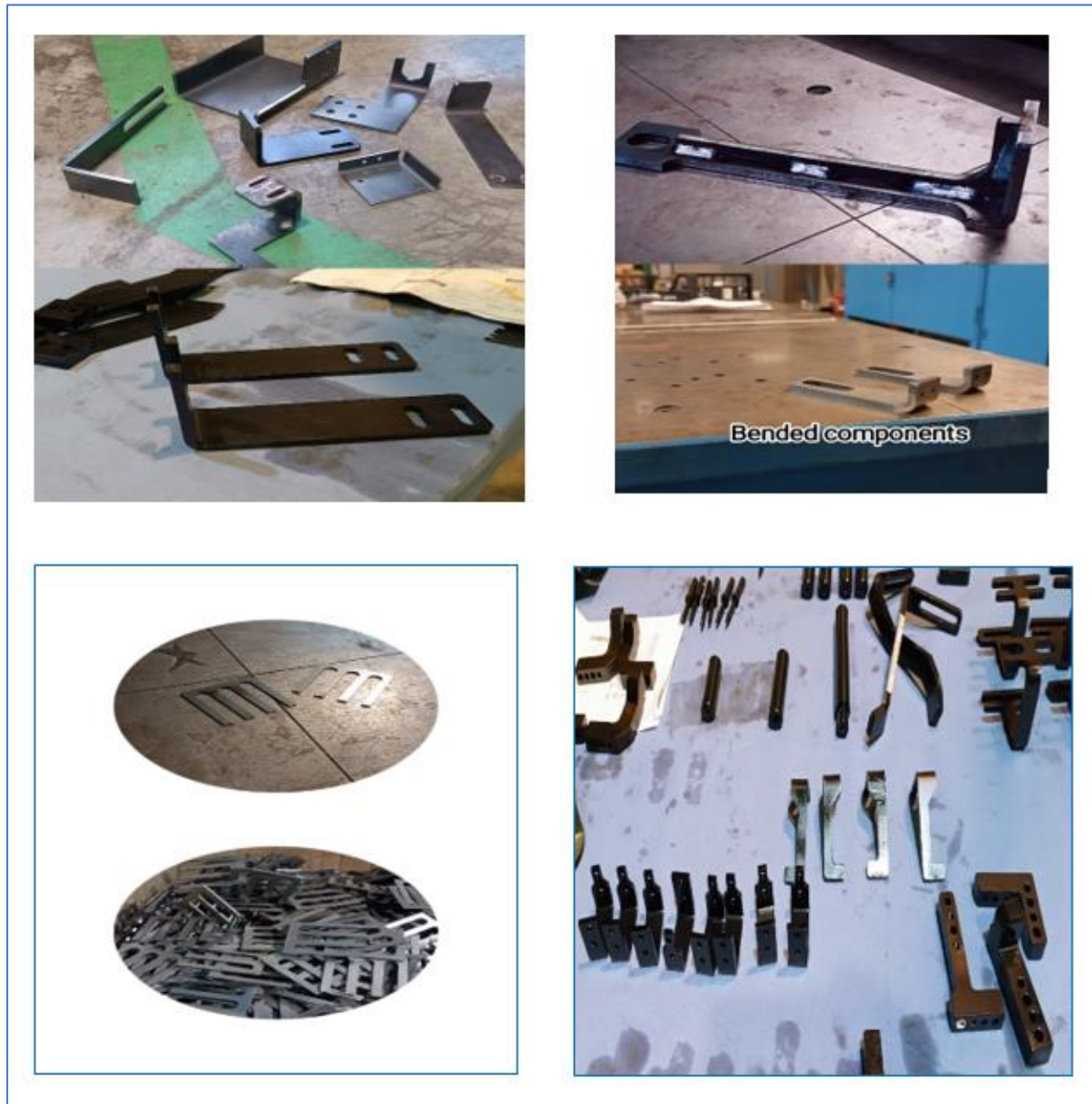
Figure 24: Example of bended Components after oxidation in bottom left, we have the shims.
