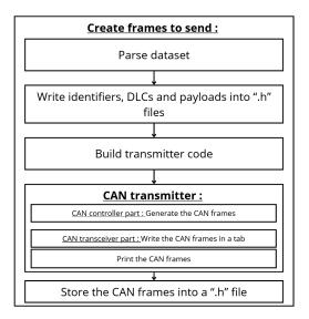
Figure 3.3: Scheme of the CAN transmitter
