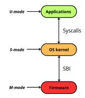
Figure 5.1: Privilege levels and interfaces of a RISC-V Linux port
