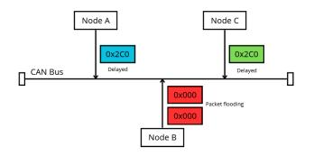
Figure 3.5: Scheme of the DoS attack
