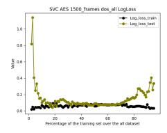
Figure B.37: DoS Log loss mean and scale dataset
