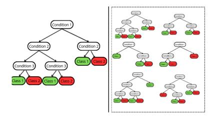
Figure 4.7: Example of a Decision tree (at left), and of a Random forest (at right)
