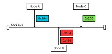
Figure 3.7: Scheme of the Impersonation attack
