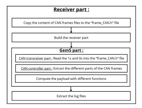
Figure 3.4: Scheme of the CAN receiver
