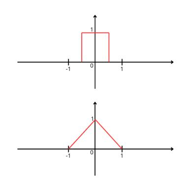
Figure 4.1: Convolution product of a rectangular function by itself
