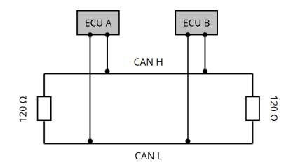
port to the CAN H and its low port to the CAN L.
