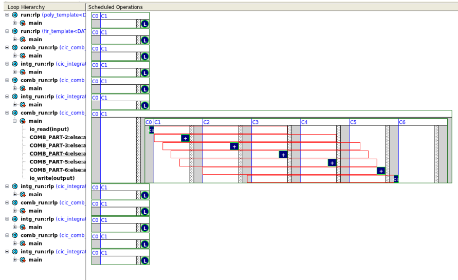
Figure 6.4: Scheduling operation of a shared adder over 4 ccs
