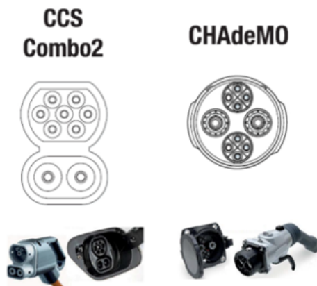
Figure 2.25: Types of DC charging connectors
