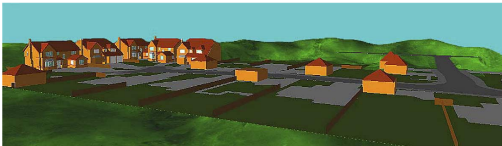
Figure 2.2: VR model assembled in a generic VR Tool using CAD house type data, and site layout data from "Visualisation in Architecture, Engineering and Construction (AEC)" [19].
