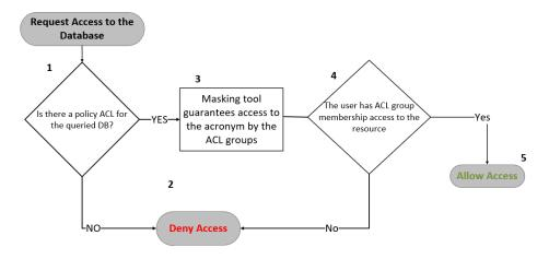
Figure 5.4: Flow of the ACL implementation
