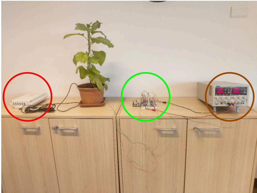
Figure 5.4: Zoom on the experimental setup which comprehends the WAPPSEN system (comprising the TEROS 21 Gen 2 sensor properly installed into the soil in the plant pot [64, 66]) on the leftmost part of the rack (in the red circle) and the CPX200D bench-type power supply unit [48] on its rightmost part (in the brown circle), while this latter is connected to this thesis developed system on its left (in the green circle), which in turn is mounted on the tobacco plant previously exploited in Section 3.4.4 and Section 3.4.5.
