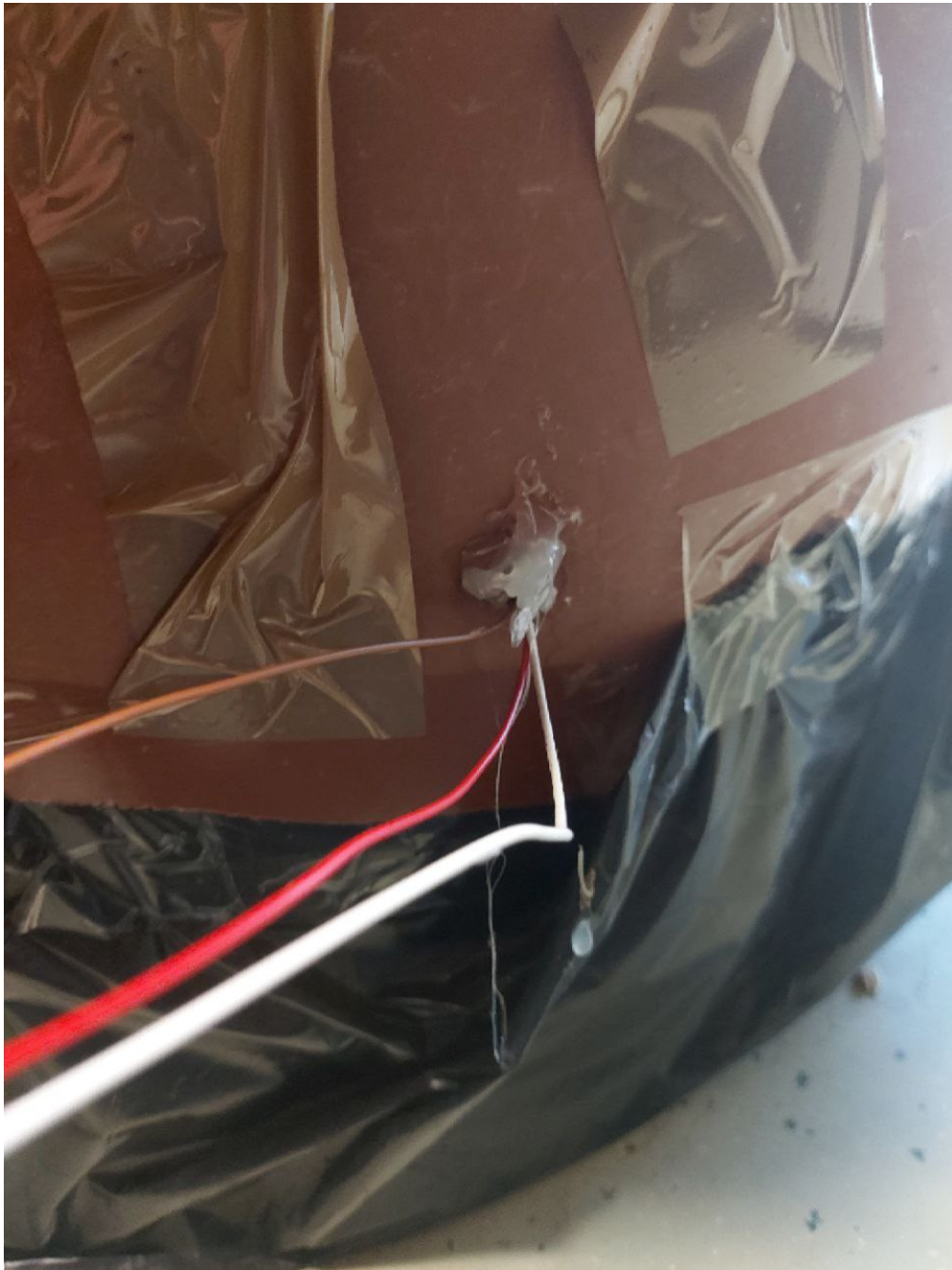
Figure 2.7: Zoom of the wires connected to the exploited electrodes (white wire associated to the zinc mesh grid, brown wire related to the copper spiral wire and red wire linked to the aluminum plate) and exiting through a thereafter-sealed hole at the bottom of the pot in PMFC 2.
