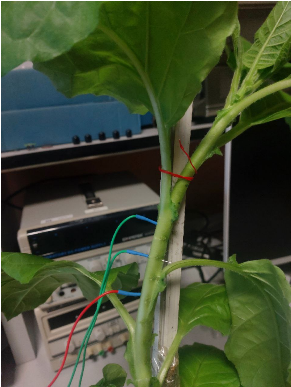
Figure 3.38: Zoom on the surgical needles employed in the characterization of the system related to a living tobacco plant.
