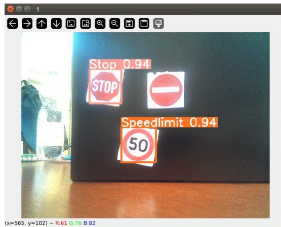
Figure 5.17: Detection of Stop and Speed Limit signals near a sign similar in shape and color
