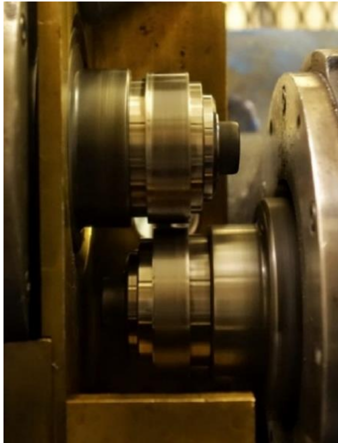
Figure 3.7: Two discs of a twin-disc tribometer in contact. Taken from “Towards a Standard Approach for the Twin Disc Testing of Top-Of Rail Friction Management Products” [50].
