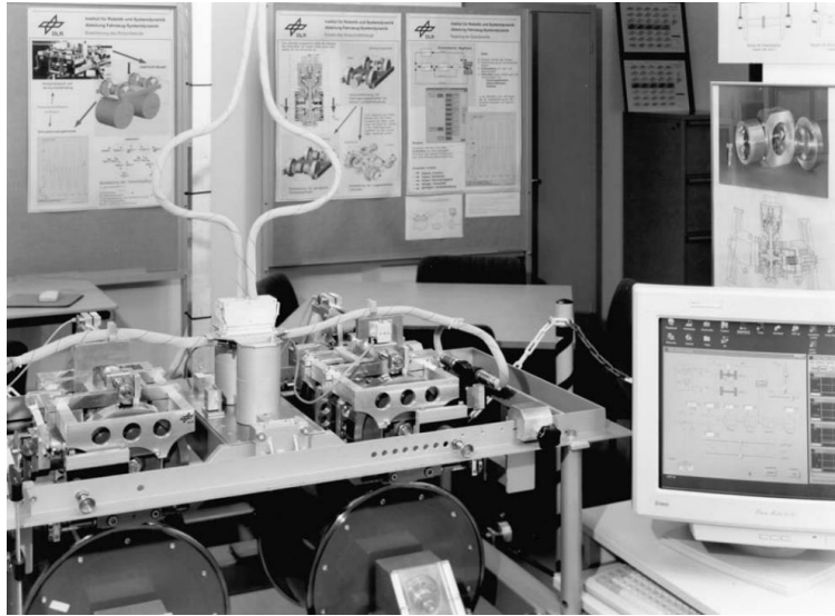
Figure 3.4: The 1/5-scale DLR roller rig developed by Jachinski et al. [44]. Taken from: “The application of roller rigs to railway vehicle dynamics” by Jaschinski, A., Chollet, H., Iwnicki, S., Wickens, A. & Von Würzen, J.
