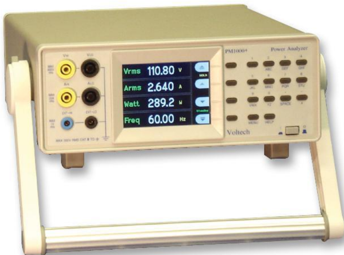
Figure 51. Voltech PM1000+ power analyzer, adapted from [95]
