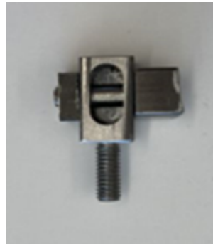
Figure 3.2. SSRT adapting tool. Screw used to stretch the wire.
