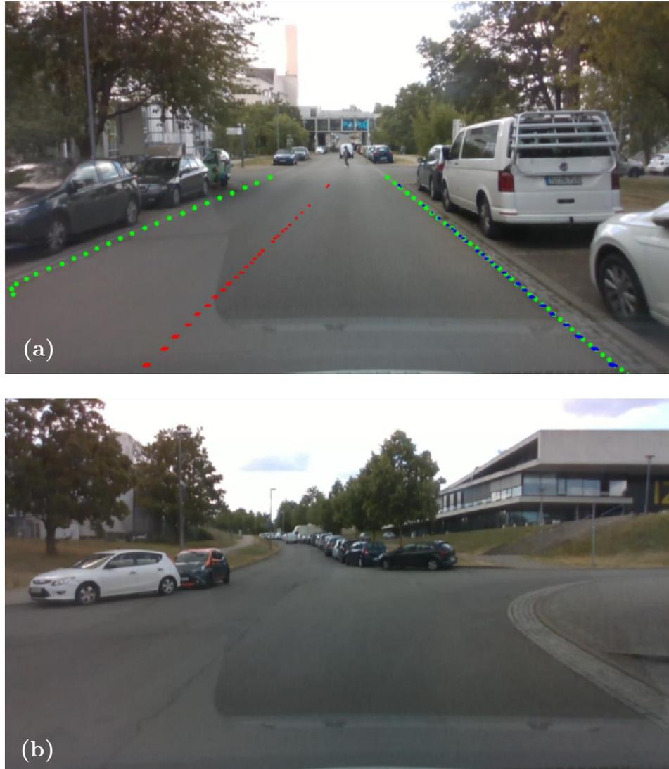
**Figure 2.5:** different behavior of the lane recognition algorithm in correspondence of a straight road (a) and intersection (b)
