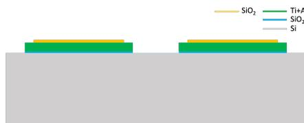
**Figure 3.24:** Wafer section after PR stripping.
