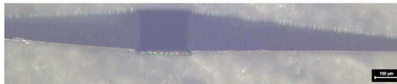
**Figure 4.25:** Optical microscope inspection of the released probe with 30  $\mu\text{m}$  trench.
