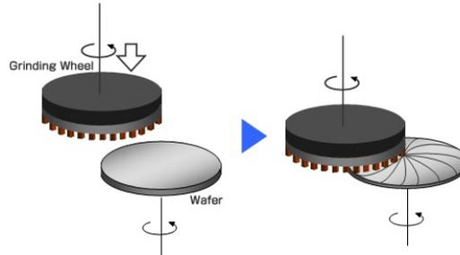
**Figure 3.25:** Grinding mechanism [68].
