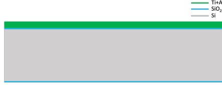
**Figure 3.6:** Wafer section after metal deposition
