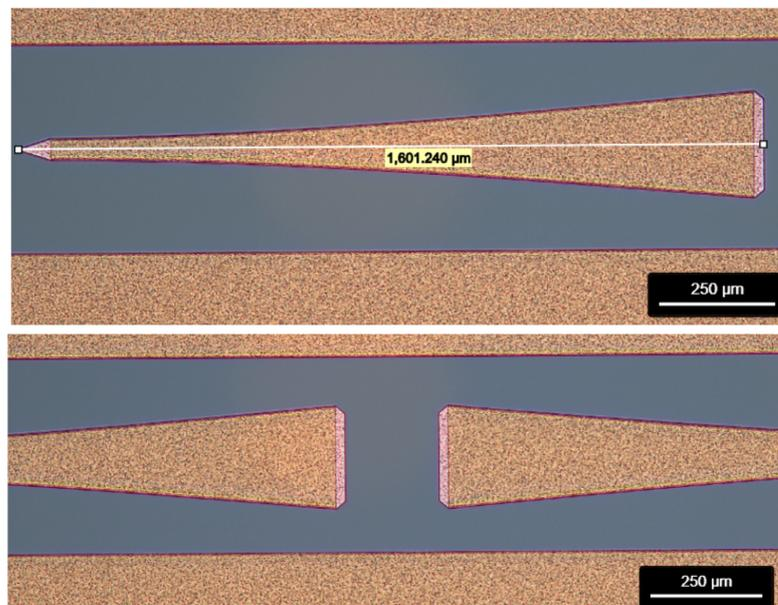
**Figure 4.3:** Probes after SiO<sub>2</sub> photolithography.
