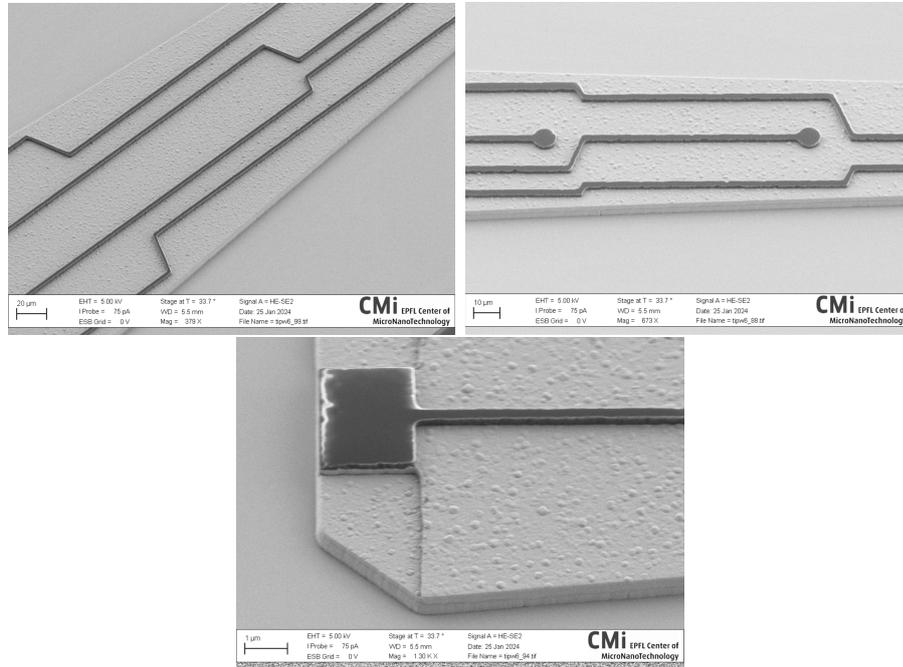
**Figure 4.27:** SEM images before the etching of the recording layer.
