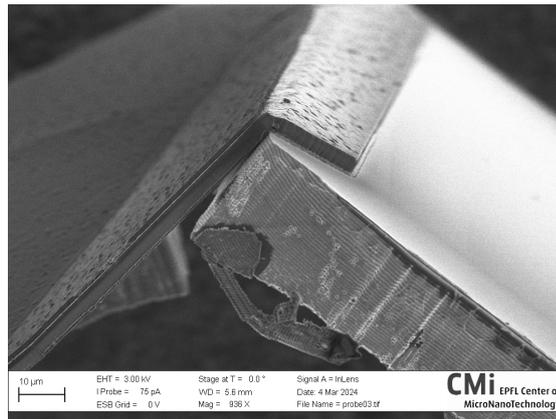
**Figure 4.31:** Optical microscope inspection of the released and bent probe with 30 μm trench.
