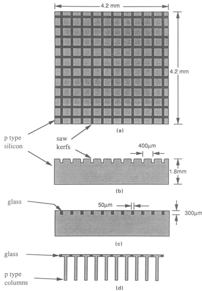
**Figure 2.2:** Silicon die illustration: A) top view, displaying perpendicular rows of incised grooves on the surface; B) profile view of the die with 50  $\mu\text{m}$  grooves; C) incorporating molten glass into the grooves and smoothing the surface; D) creating columns in the die through a diamond dicing saw. Reprinted from [29]
