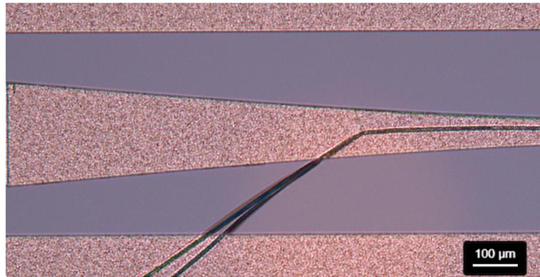
**Figure 4.2:** Example of unsuccessful stripping with photo resist residuals.
