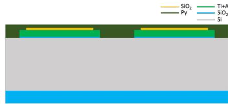
**Figure 3.29:** Wafer section after Parylene-C etching on backside.
