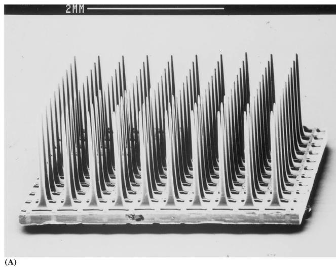
**Figure 2.3:** SEM image of Utah Intracortical Electrode Array. Reprinted from [30]
