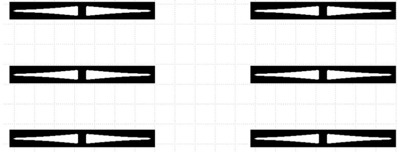
**Figure 3.11:** Design for Al photolithography.
