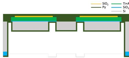
**Figure 3.40:** Wafer section after backside Parylene coating.
