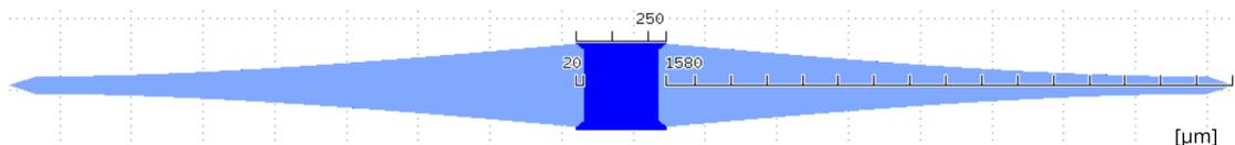
**Figure 3.3:** Illustration of the probe design with respective dimensions.
