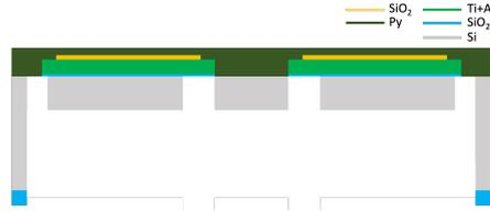
**Figure 3.39:** Wafer section after second deep silicon etching.
