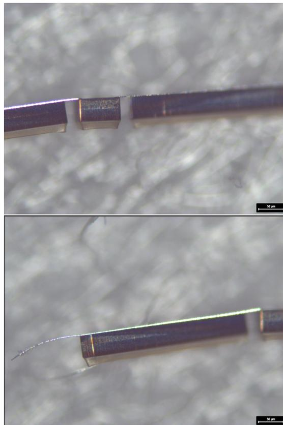
**Figure 4.22:** Optical microscope inspection of the released probe with 70  $\mu\text{m}$  trench.
