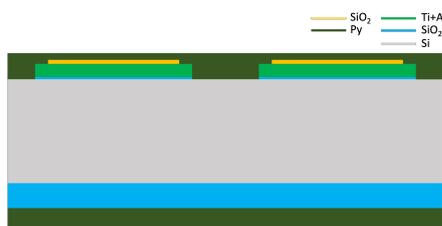
**Figure 3.28:** Wafer section after Parylene-C coating.
