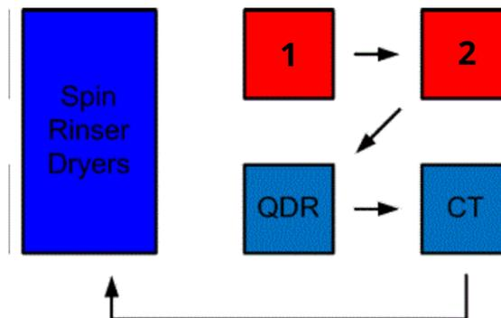
**Figure 3.18:** UFT Resist wetbench sequence: 1 & 2: baths of REM1165 at 70°C (min); QDR: Quick Dump Rinse (rough rinsing); CT: Cascade Tank (fine rinsing) [63].
