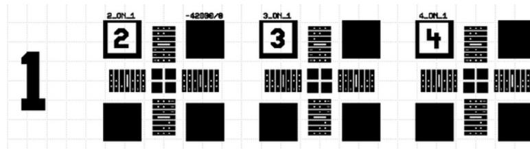
**Figure 3.12:** Alignment crosses for the first photolithography.
