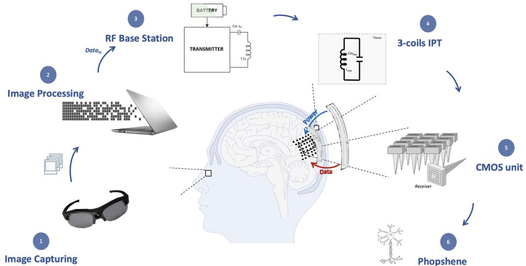
**Figure 1.2:** Schematic representation of the concerned visual prosthesis.
