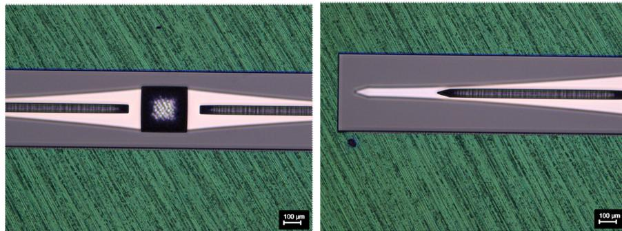
**Figure 4.21:** Optical microscope inspection at the end of the last deep silicon etching step.
