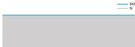
Figure 3.5: Wafer section after Wet Oxidation
