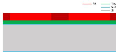
Figure 3.10: Wafer section after PR coating.
