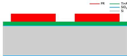
**Figure 3.14:** Wafer section after PR development.
