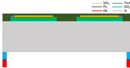
**Figure 3.32:** Wafer section after SiO<sub>2</sub> etching.
