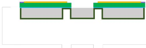
**Figure 3.41:** Wafer section after probes release.
