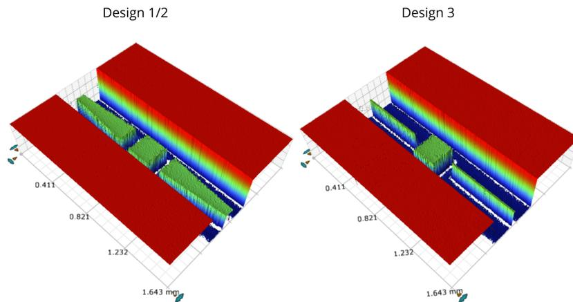
**Figure 4.20:** Optical profilometer 3D evaluation for both designs.
