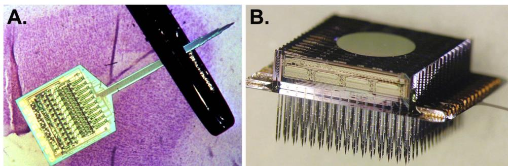
**Figure 2.7:** (A) Illustration of a four-tine fork featuring two rows of microelectrodes on each prong. The probe base's contact pads serve for interconnections or cable assemblies. (B) A NeuroProbe array in three dimensions, featuring multiple recording sites connected to a pliable ribbon cable. Taken from [25]
