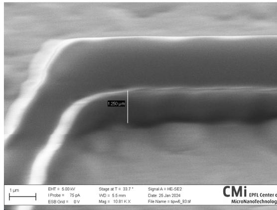
**Figure 4.26:** SEM image before the etching of the recording layer.
