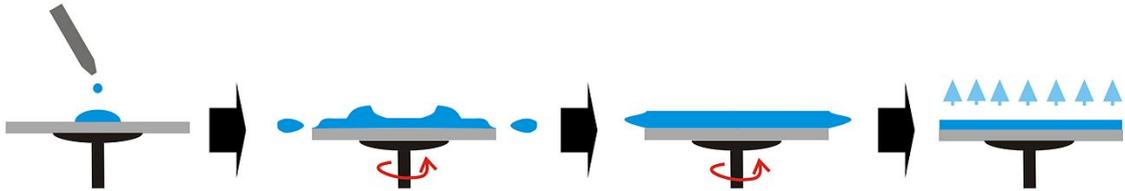
**Figure 3.8:** Spin coating technique [54].
