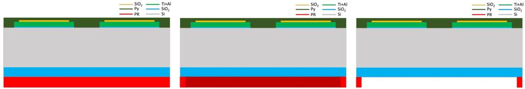
**Figure 3.31:** Wafer section after: a) PR coating; b) Exposure; c) PR development.
