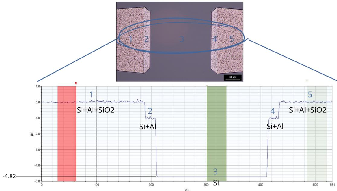
**Figure 4.5:** Probes profile obtained from optical profilometer after  $\text{SiO}_2$  etching.
