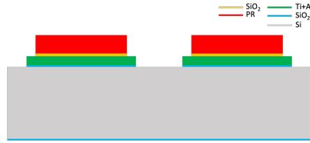
**Figure 3.22:** Wafer section after SiO<sub>2</sub> etching.
