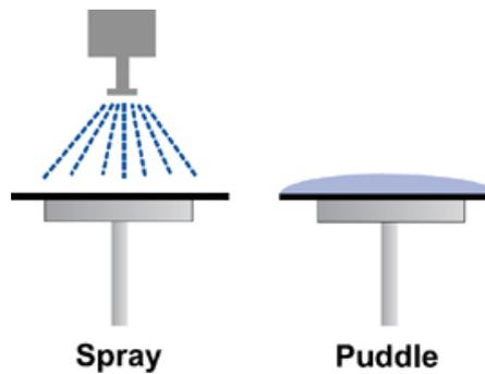
**Figure 3.15:** Illustration of spray dispense and puddle development method.
