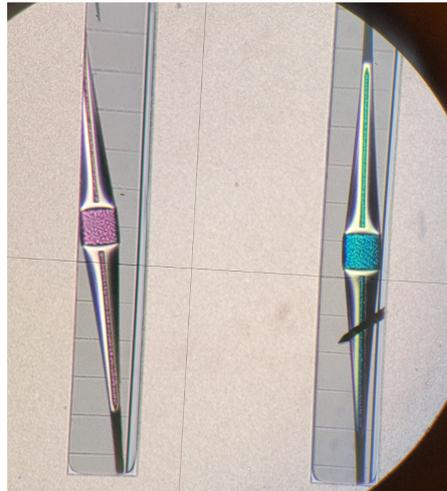
**Figure 4.24:** Optical microscope inspection of the released probes inside the cavities.
