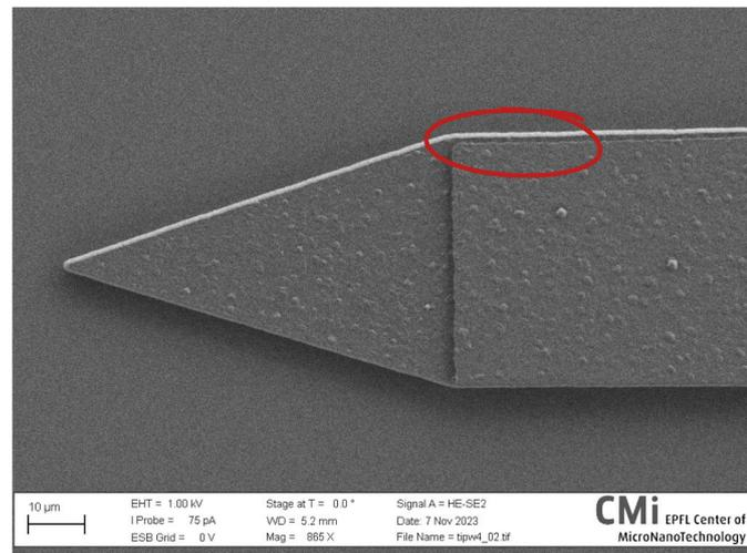
**Figure 4.6:** Tip morphology obtained by SEM analysis.
