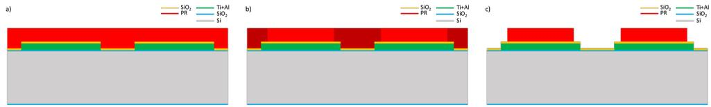
**Figure 3.21:** Wafer section after: a) PR coating; b) Exposure; c) PR development.
