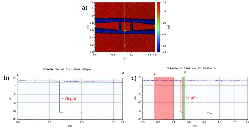
**Figure 4.15:** Optical profilometer profile evaluation after the first deep silicon etching step. a) probe backside design, b) depth x-profile, c) depth y-profile.
