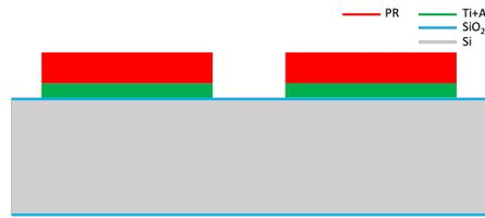
**Figure 3.16:** Wafer section after Al etching.
