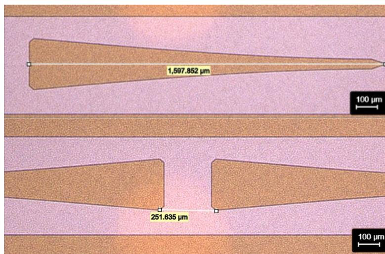
**Figure 4.1:** Probes after Aluminum photolithography.
