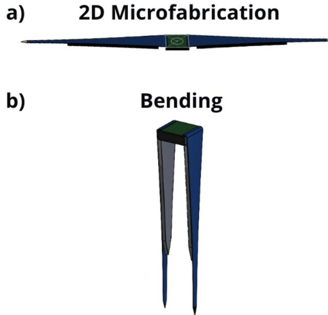
**Figure 3.1:** Schematic representation illustrating the final fabrication result in 2D a) and subsequent to the bending process b).
