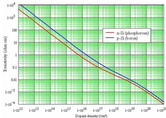
**Figure 3.2:** Relationship between Dopant Concentration and Resistivity in Silicon. Reprinted from [41].
