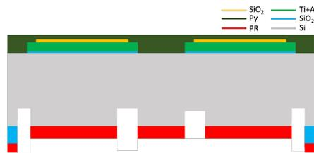
**Figure 3.36:** Wafer section after first deep silicon etching.
