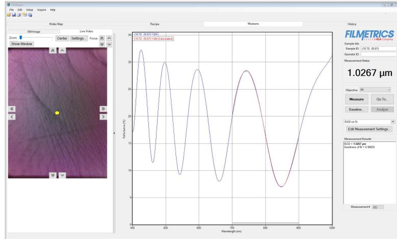
**Figure 4.10:**  $\text{SiO}_2$  thickness in the center measured with *Filmetrics F54*.
