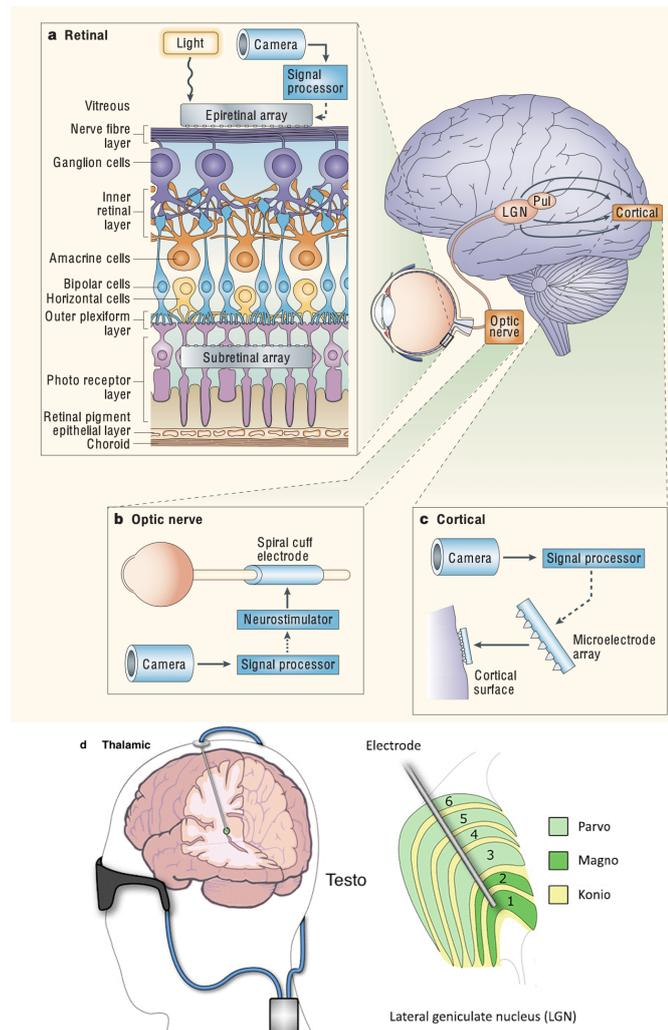
**Figure 1.1:** Overview of a) Retinal, b) Optic nerve, c) Cortical and d) Thalamic implants. Reprinted from [7] and [8]
