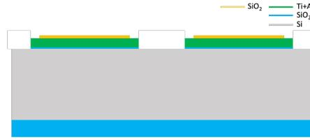
**Figure 3.27:** Wafer section after SiO<sub>2</sub> deposition.
