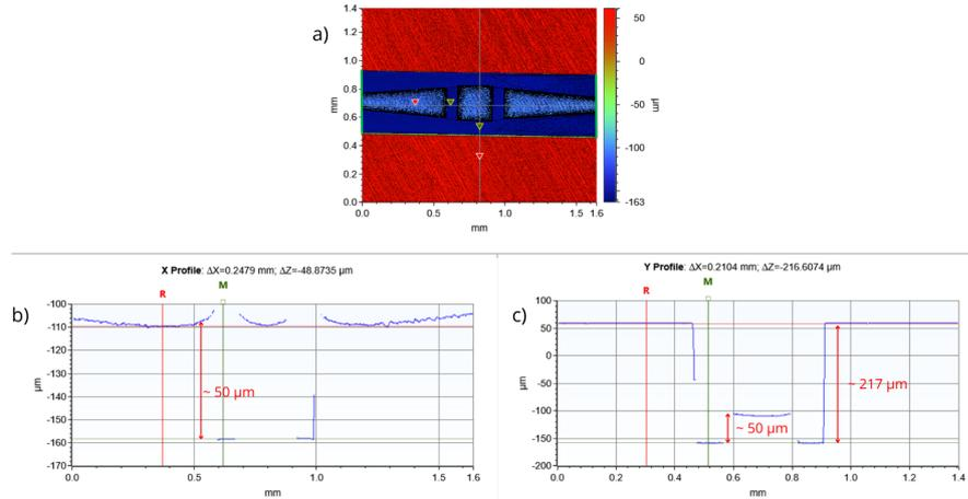
**Figure 4.18:** Optical profilometer profile evaluation at the end of the last deep silicon etching step for designs 1 and 2. a) probe backside design, b) depth x-profile, c) depth y-profile.
