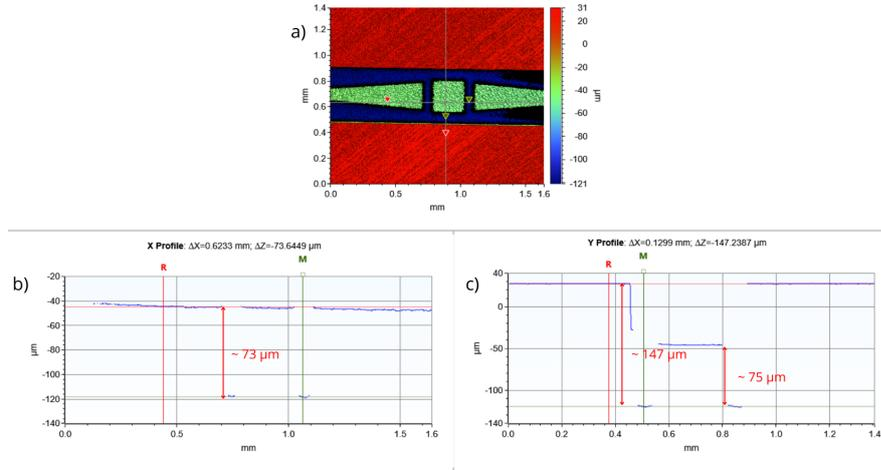
**Figure 4.17:** Optical profilometer profile evaluation after the first iteration of the last deep silicon etching step. a) probe backside design, b) depth x-profile, c) depth y-profile.
