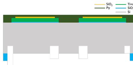
**Figure 3.38:** Wafer section after PR stripping.
