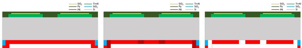
Figure 3.35: Wafer section after: a) PR coating; b) Exposure; c) PR development.
