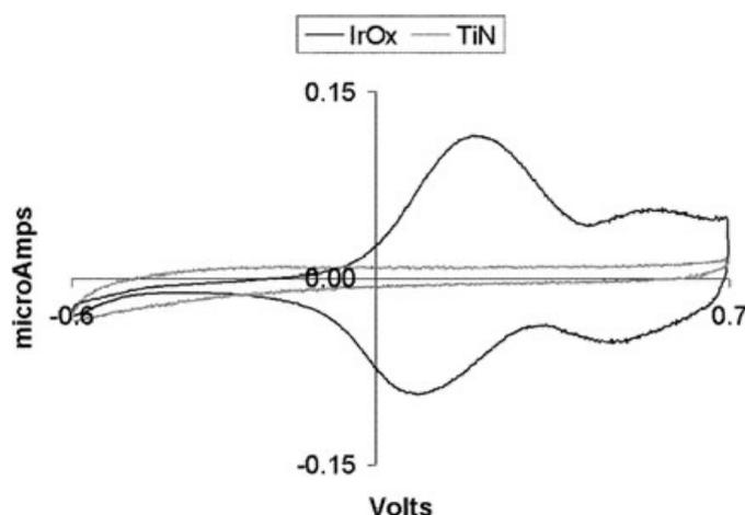
**Figure 2.1:** Cyclic voltammogram for IrOx and TiN, the reference electrode was a saturated calomel electrode. Reprinted from [22]
