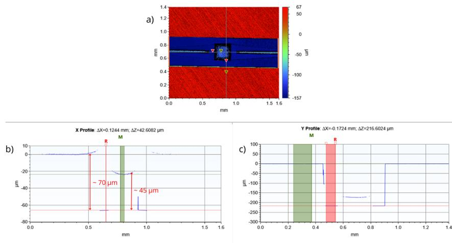
**Figure 4.19:** Optical profilometer profile evaluation at the end of the last deep silicon etching step for design 3. a) probe backside design, b) depth x-profile, c) depth y-profile.
