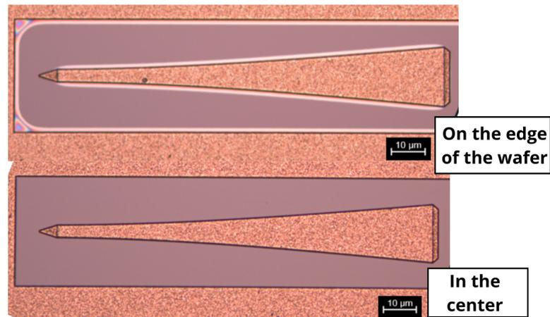
**Figure 4.11:** Parylene adhesion inspection, comparison between structures at the edge and in the center.
