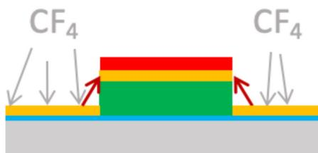
**Figure 4.7:** Scattering of ions during etching.
