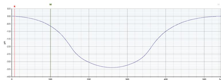
Figure 4.9: Thickness evaluation after 15  $\mu$ m PR coating using mechanical profilometer.
