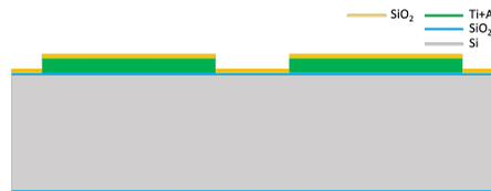
**Figure 3.19:** Wafer section after SiO<sub>2</sub> deposition.
