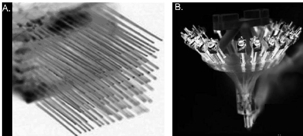
**Figure 2.4:** (A) Handcrafted penetrating microelectrode array assembled from several insulated wires with trimmed ends. (B) Microwire array designed for long-term utilization in small animal experiments. Reprinted from [25]
