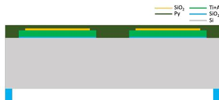
**Figure 3.33:** Wafer section after PR stripping.
