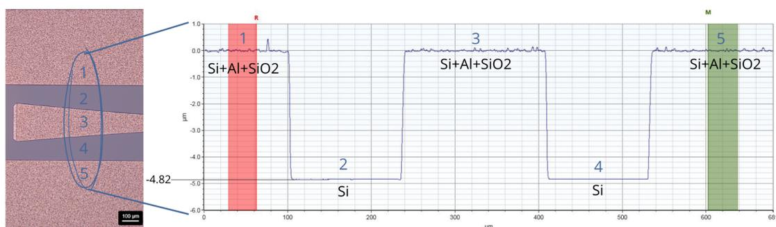
**Figure 4.4:** Probes profile obtained from optical profilometer after SiO<sub>2</sub> etching.
