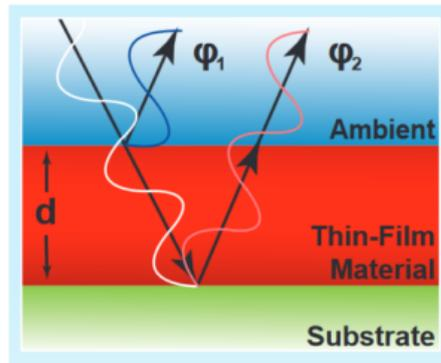
**Figure 3.23:** *Filmetrics F54* working principle [67].
