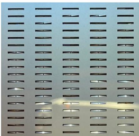
**Figure 4.23:** Optical microscope inspection of the cavities after probes release.
