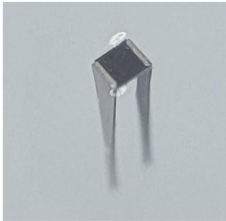
**Figure 4.33:** Optical microscope photo of the bent probe after implantation.
