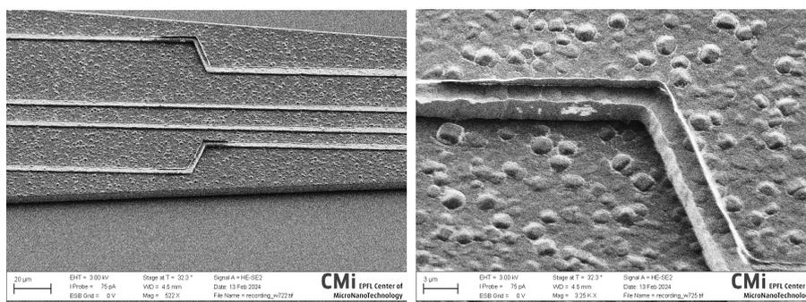
**Figure 4.28:** SEM images after the etching of the recording layer.
