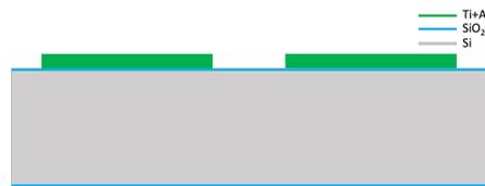
**Figure 3.17:** Wafer section after PR stripping.
