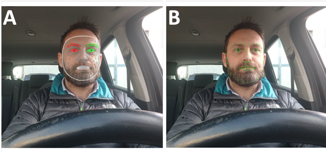
Figure 6.5: Figure A depicts the image of the driver in the car after processing with Mediapipe, while Figure B shows the image obtained with Dlib.
