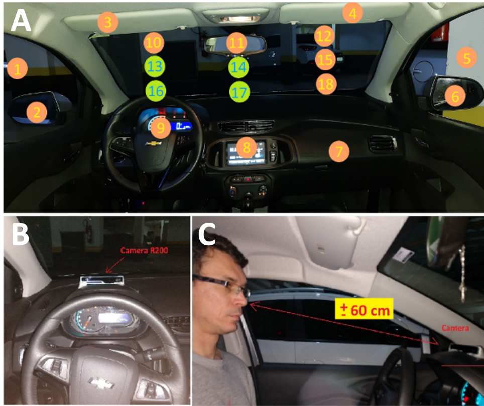
Figure 5.2: In Figure A, the key points where the driver gazes during driving are highlighted, based on the DG-Unicamp dataset [95]. Point 19 is not displayed, indicating a moment when the driver has closed eyes. Figure B shows the driver’s view, with the camera position above the tachometer. Figure C highlights the approximate distance of about 60 cm between the camera and the driver. Source [95].
