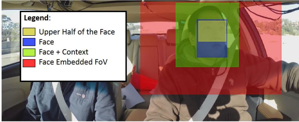
Figure 4.3: Different cropped regions from the input image used for CNN training, with each cropped region colored for clear distinction. Source [80].
