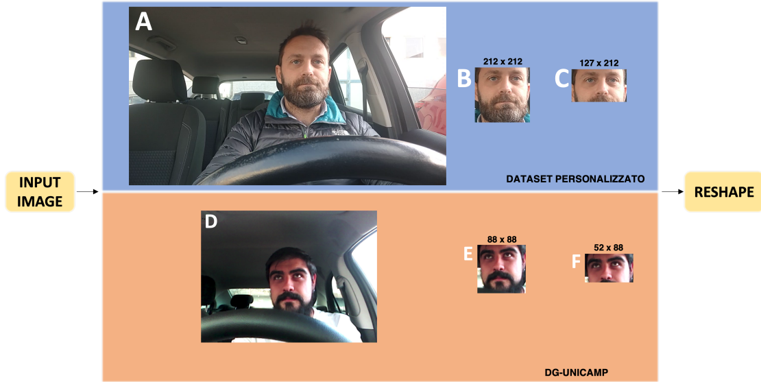
Figure 6.3: The figure illustrates various pre-processing methodologies applied to both images from the custom dataset (A, B, C) and those from the DG-UNICAMP dataset (D, E, F), both intended for the CNN. The input images from the custom dataset maintain a resolution of 1280x720 pixels, while those from DG-UNICAMP are 240x320 pixels. Images A and D represent the originals without any pre-processing; images B and E feature the face cropped using Mediapipe [97] (see Section 6.3.1), while images C and F show a type three pre-processing, with the upper face area cropped by 60%. Subsequently, all images are uniformly resized to 224x224 pixels. The difference in resolution between the images from the custom dataset and those from the DG-UNICAMP dataset is evident following pre-processing.
