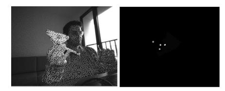
**Figure 6.5:** Realsense Depth Camera and Kinect Spherical Marker Acquisition comparison
