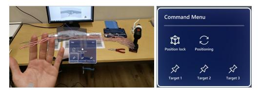
Figure 3.6: Command Menu displayed in AR user interface
