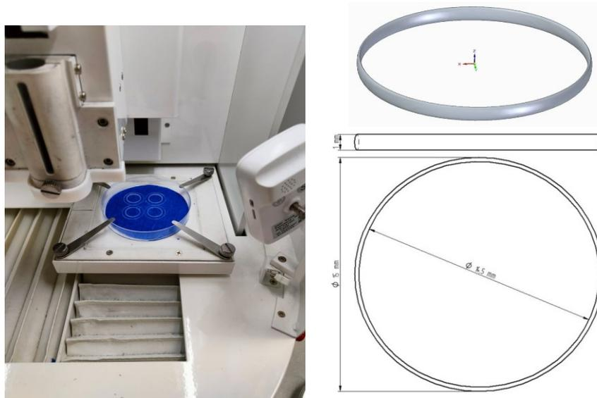
*Figure 22. PCL custom-made ring CAD model and fabrication*
