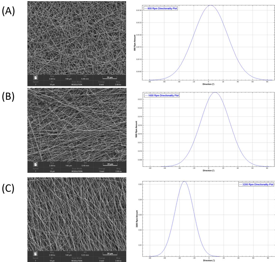
**Figure 7.** SEM image of a membrane spun at 800 (A), 1600 (B) and 3200 (C) rpm and its directionality Plot
