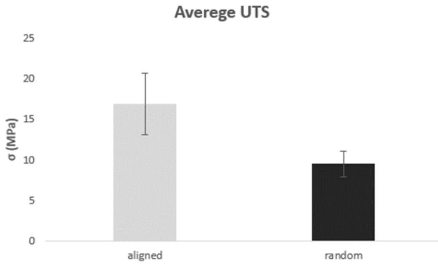
*Figure 10. Average UTS comparison of random and aligned fibers*
