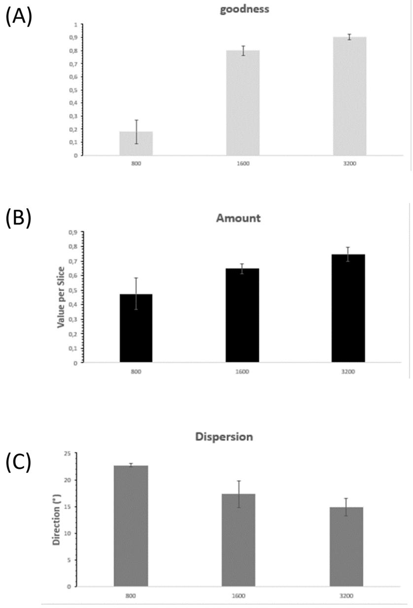
Figure 8. Gaussian goodness (A), fibers amount (B) and fiber dispersion (C) comparison between 800, 1600 and 3200 rpm
