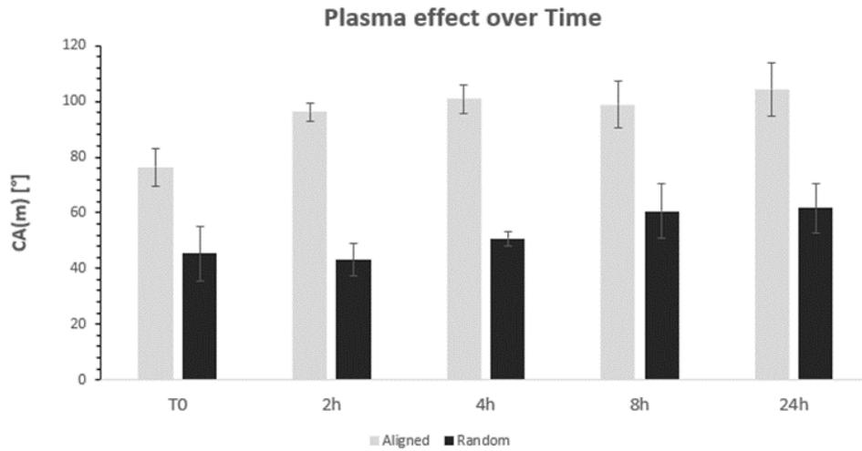
Figure 14. Comparison between aligned and random fibers contact angle trend after different time steps
