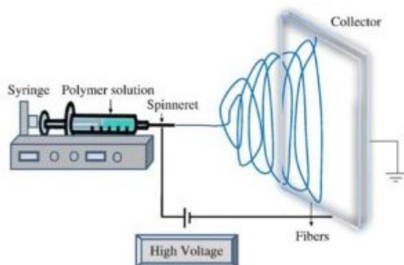
*Figure 3. Electrospinning process graphic scheme*
