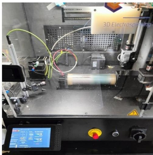
*Figure 4. Electrospinning process using rotating collector*
