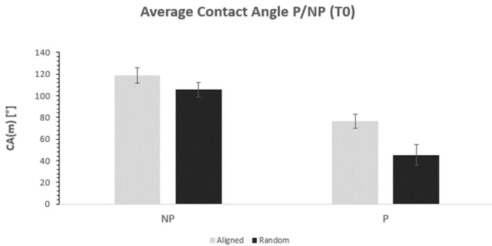
Figure 13. Average contact angles between treated and not treated membranes comparison
