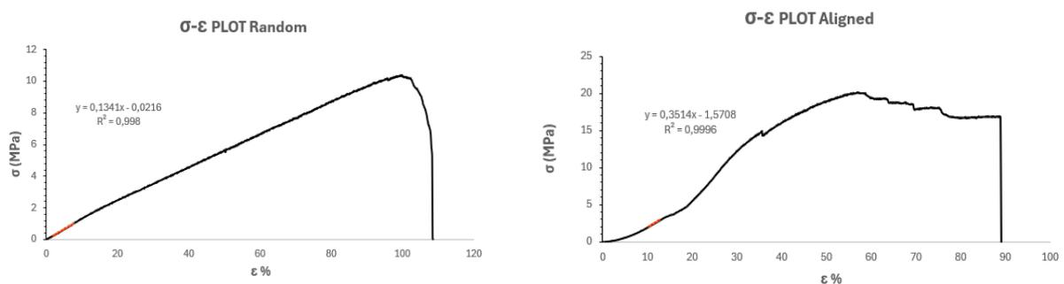
Figure 9. Average strain stress curves for random and aligned samples
