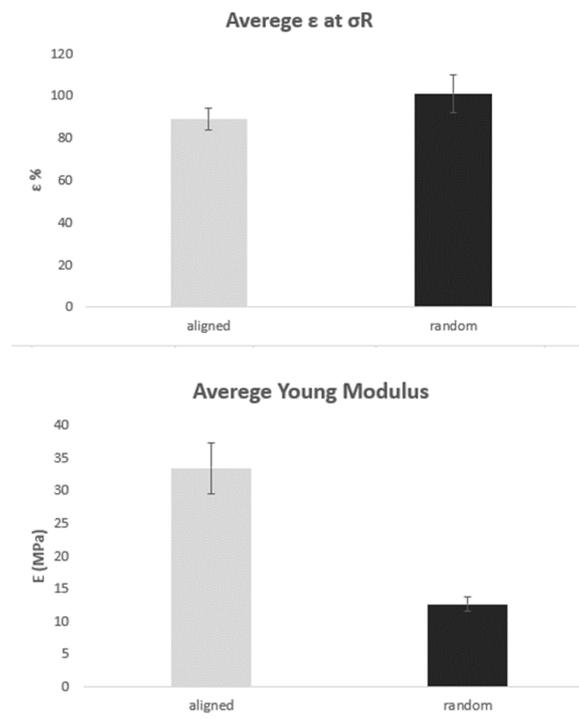
*Figure 11. Average deformation at break and Young modulus comparison between random and aligned fibers*
