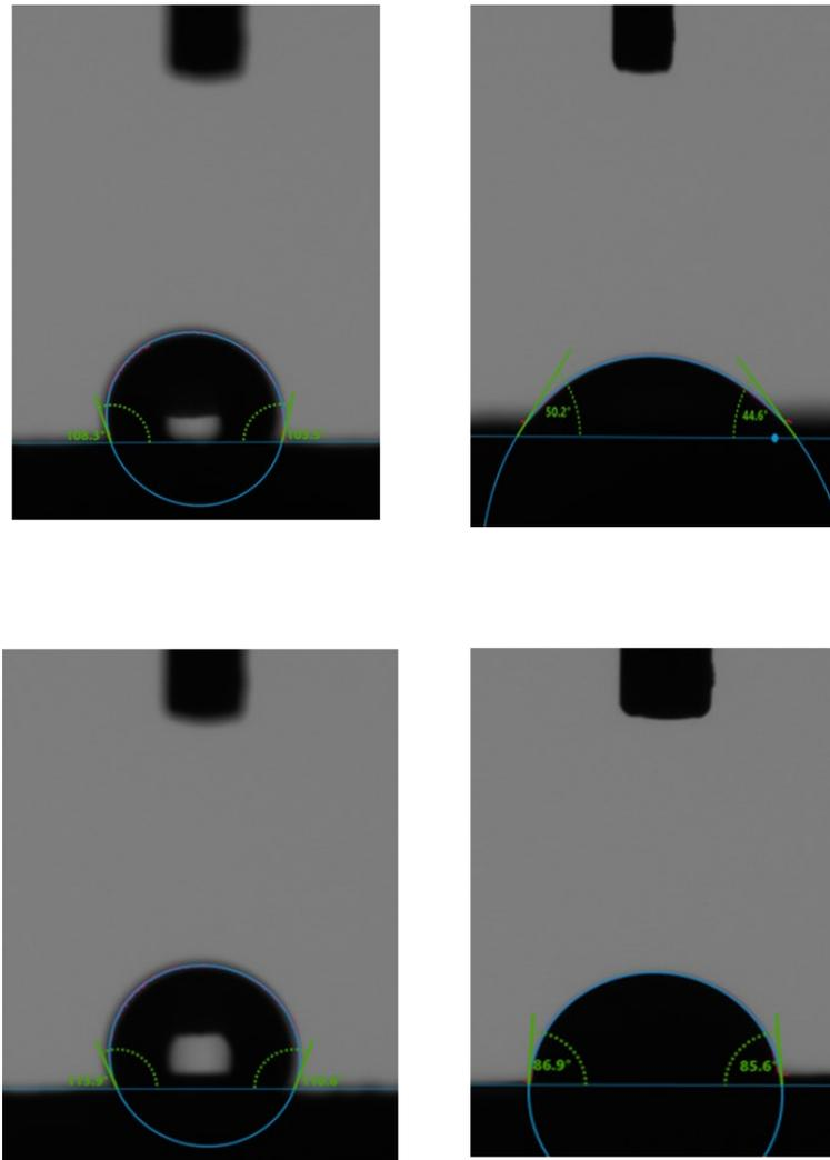
Figure 12. Random and aligned fibers samples before and after the plasma treatment images
