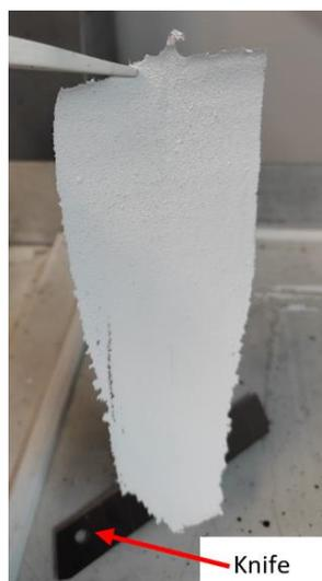
Figure 24 - Slurry casted electrolyte tape detached from the glass support
