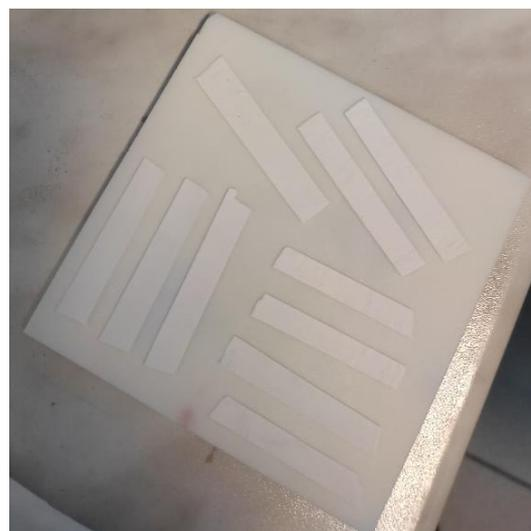
Figure 25 - Slurry casted electrolytes
