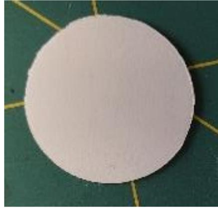
*Figure 11 - Compressed powder based electrolyte*
