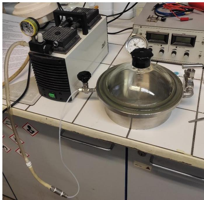
*Figure 56 - Vacuum drier connected to a vacuum pump*
