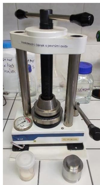
Figure 9 - Hydraulic press, mold, and paper sheets
