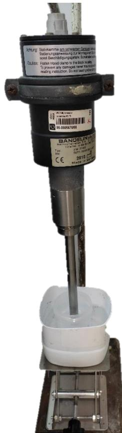
*Figure 59 - Ultrasound horn pre-treatment*
