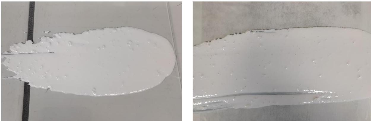
*Figure 60 - Casted tapes plenty of clumps after ultrasound horn pre-treatment*
