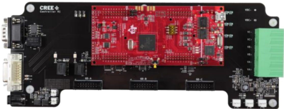
Figure 1.3: Picture of the existing TI control board[1].
