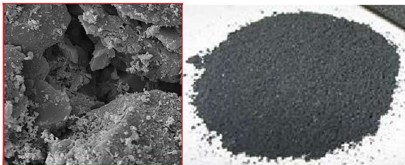
Figura 28 - Industrial multiwall carbon nanotubes
