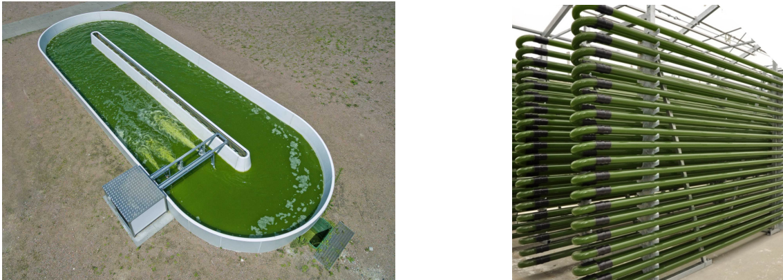
Figure 18: A raceway open pond system (on the left) and a tubular photobioreactor (on the right)
