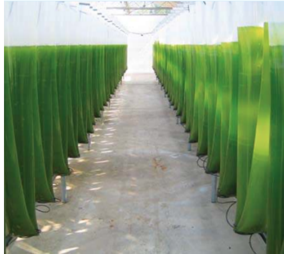
Figure 27: Hanging bags in the greenhouse at Niederaussem power station [72]
