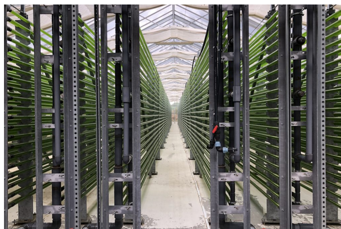
Figure 39: Partially open shading system above the PBR in Roquette Klötze GmbH & Co. KG Chlorella vulgaris cultivation plant [32]
