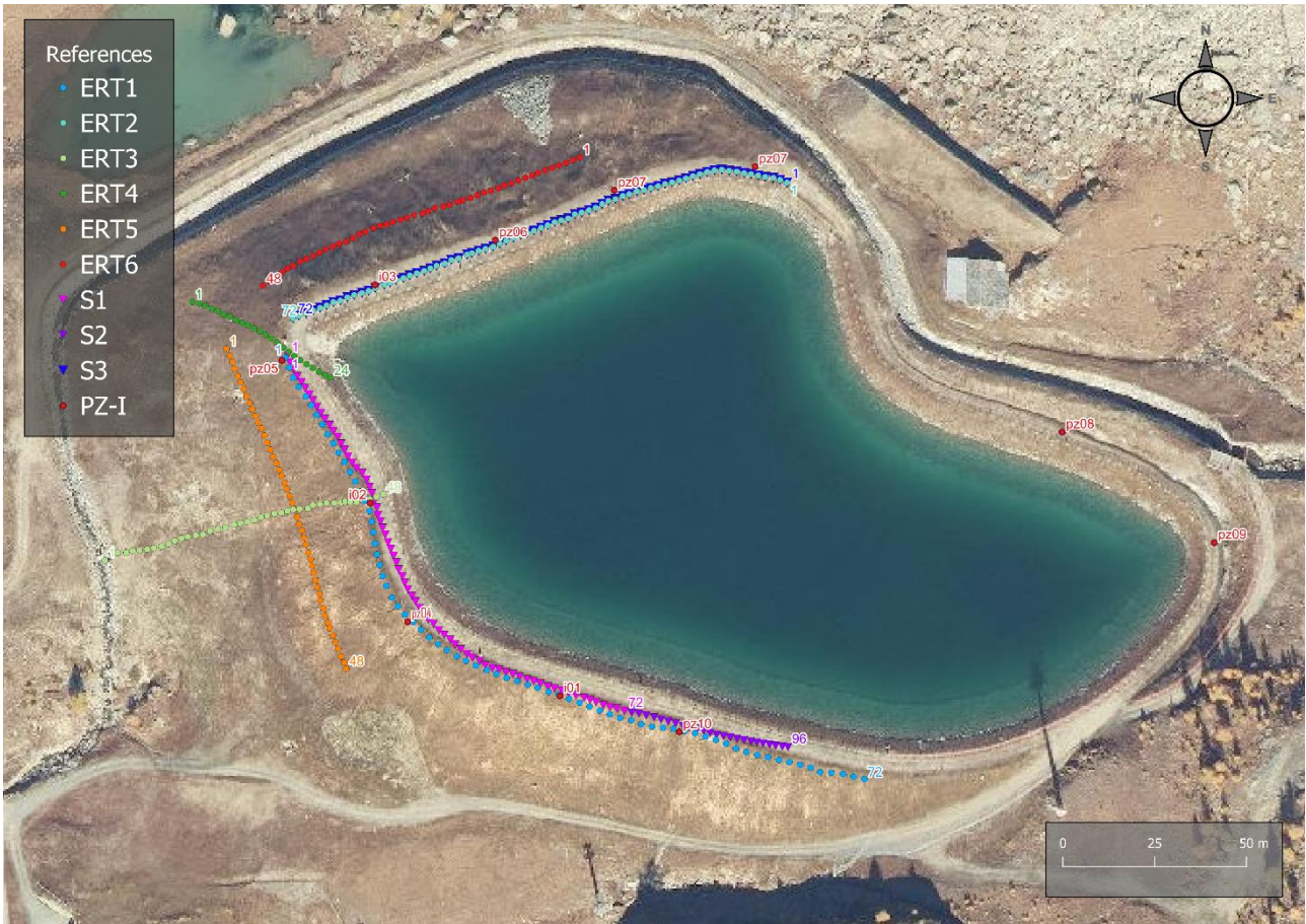
Figure 3 ERT and Seismic Surveys performed at the basing of the Fourcare Embankment to assess Thesis and Nodes Project Objectives
