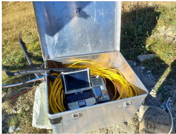
Figure 6 Laptop and resistance meter from electrical resistivity tomography survey performed in July 2023 at Fourcare dam, Valle d'Aosta.
