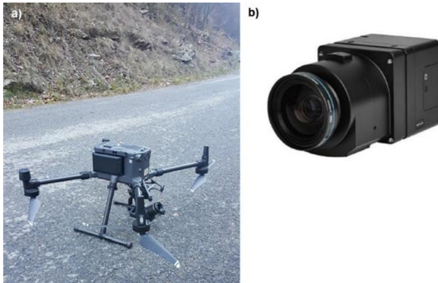
Figure 71 - Drone and camera utilized for aerial photogrammetry survey (courtesy of Maschio P.).
