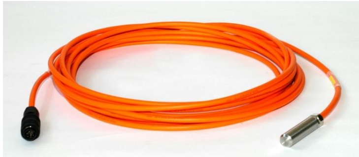
Figure 66 – Example of pressurized water-tight encapsulated sensors employed for measuring temperature in the ground, rock, or on the structure (from SOLEXPERTS).
