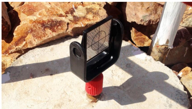
Figure 68 - A topographic target mounted on a rock mass (from SISGEO).
