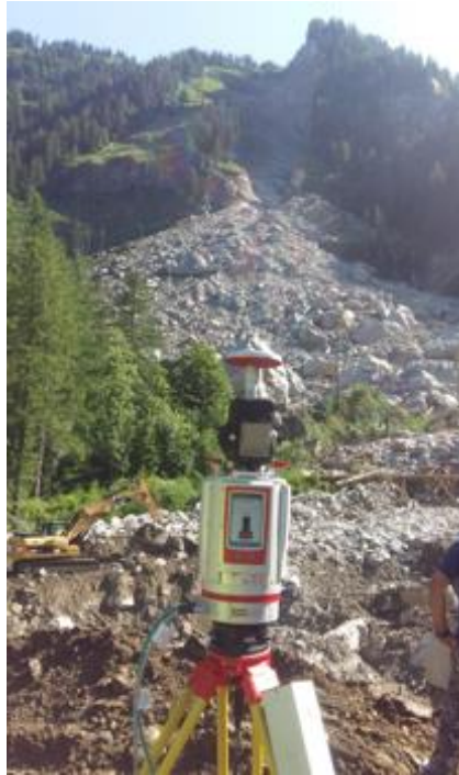
Figure 69 - LiDAR device (courtesy of Cina A.).
