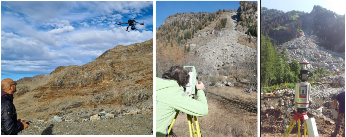
Figure 45 - a) Drone photogrammetry; b) total station; c) LiDAR (courtesy of Maschio P. and Cina A.).
