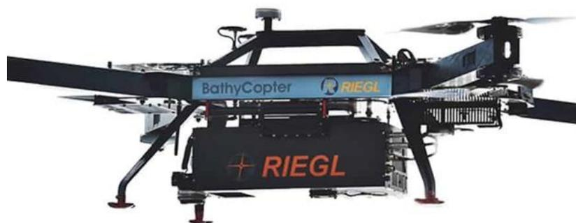
Figura 2.5, Green LiDAR BathyCopter RIEGL
